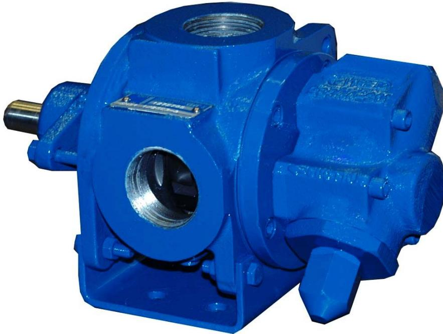
The GMS series is designed for applications in the operating ranges noted below. These units are available with head and backhead jackets (R size only) for temperature control, carbon graphite bushings for low viscosity liquids, silicon carbide bushings for wear resistance, and carbide, positive drive or packing seals for viscous sealing.
