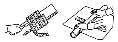
Step 1: Determine how much bulk packing will be required to fill the packing cavity, and wrap it around a rod of the same diameter as the shaft. With the packing wrapped around the rod, cut through each turn as shown.
