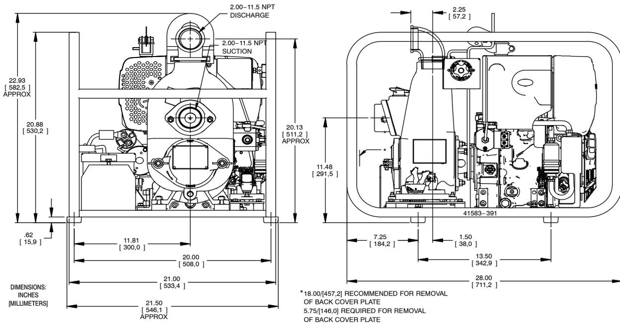
**Figure 1. Pump Model 12D1-1B30E FT4 S/G**
