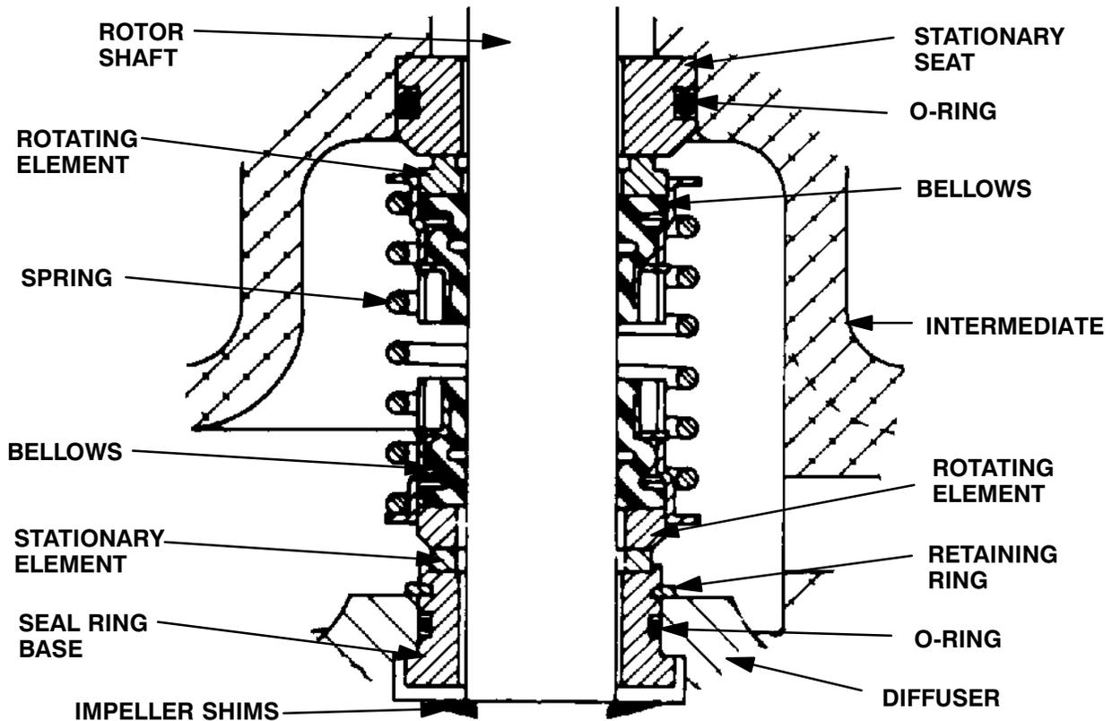
Figure 3. 10214 Seal Assembly
