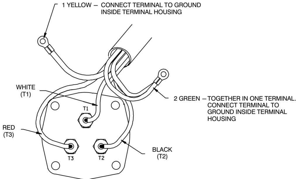
**Figure 5. Terminal Housing Wiring Connections**
