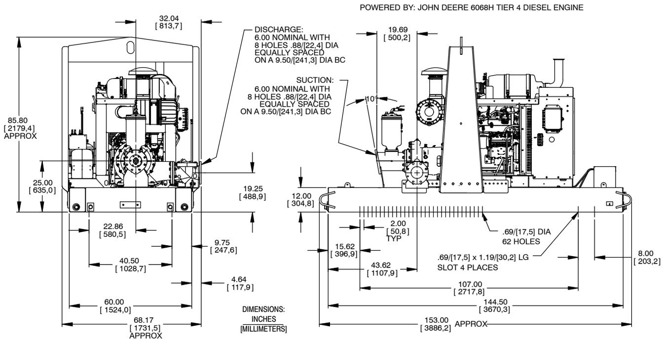
**Figure 1. Pump Model PA6B60-6068H FT4**
