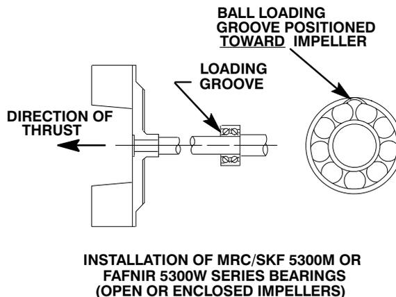
**Figure 8. Bearing Installation**
