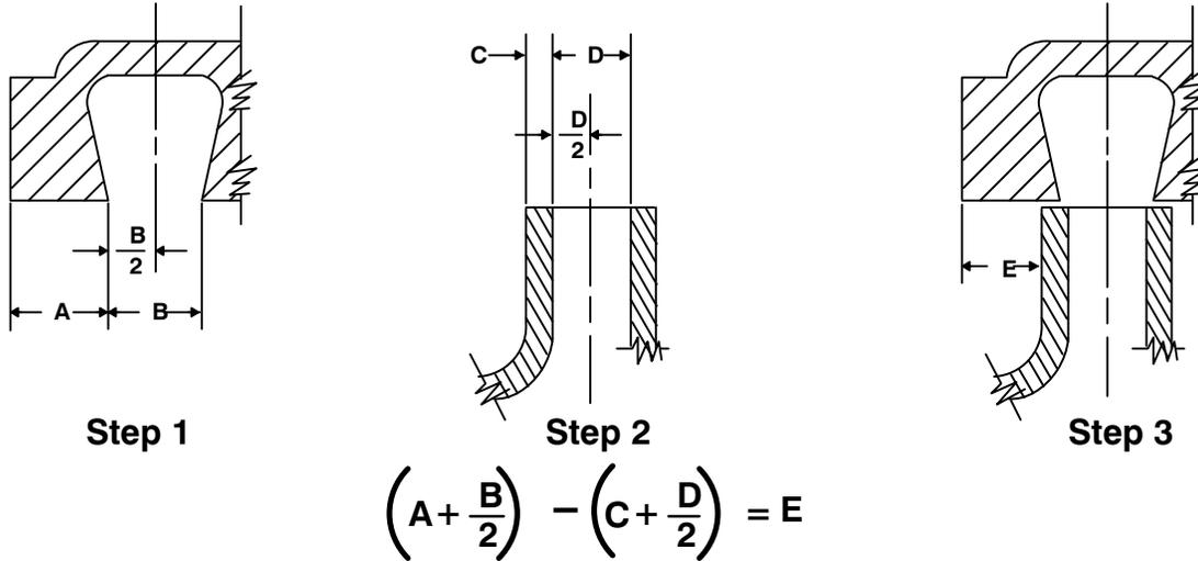
**Figure 10. Centering Impeller Within Volute Scroll**
