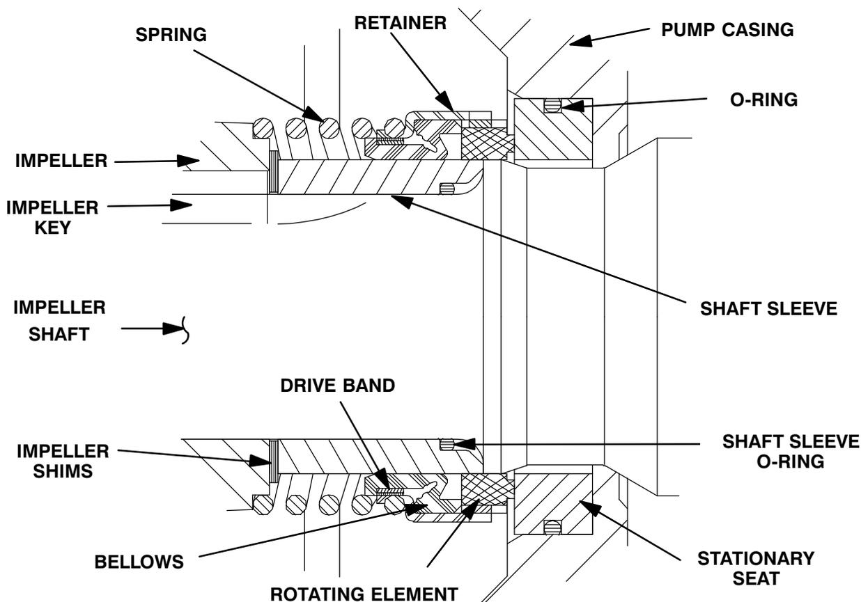
**Figure 9. Seal Assembly**
