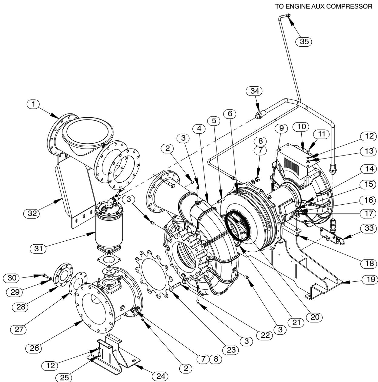
Figure 4. Pump End Assembly
