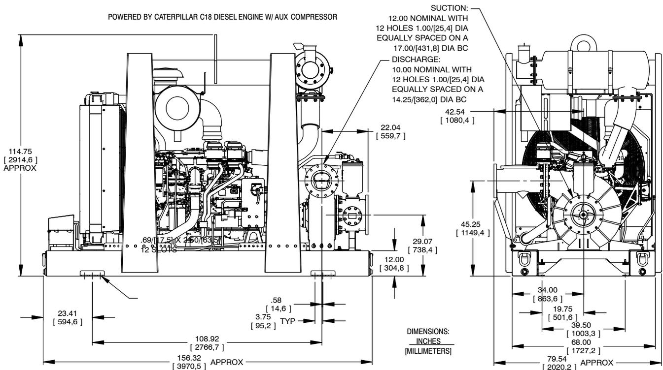
Figure 1. Pump Model PAH10A60-C18
