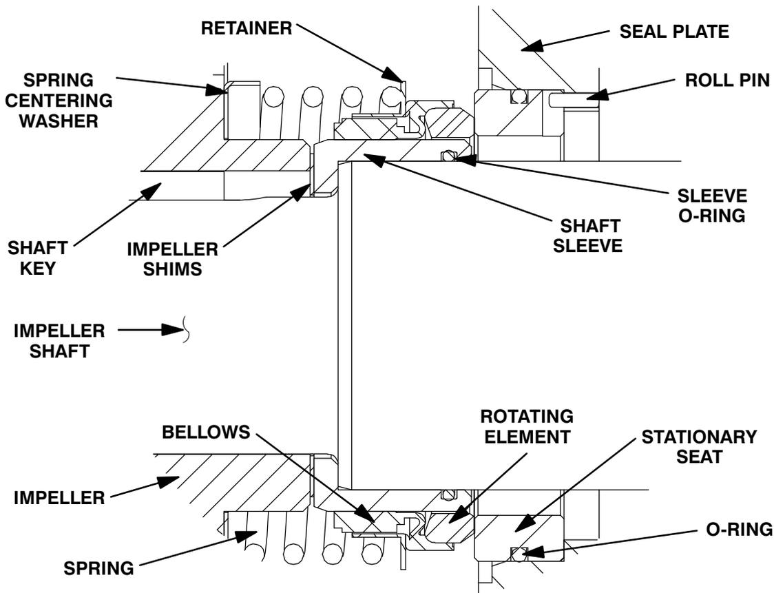
**Figure 9. Seal Assembly**
