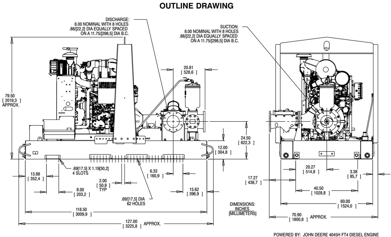
**Figure 1. Pump Model PA8E60-4045H FT4**
