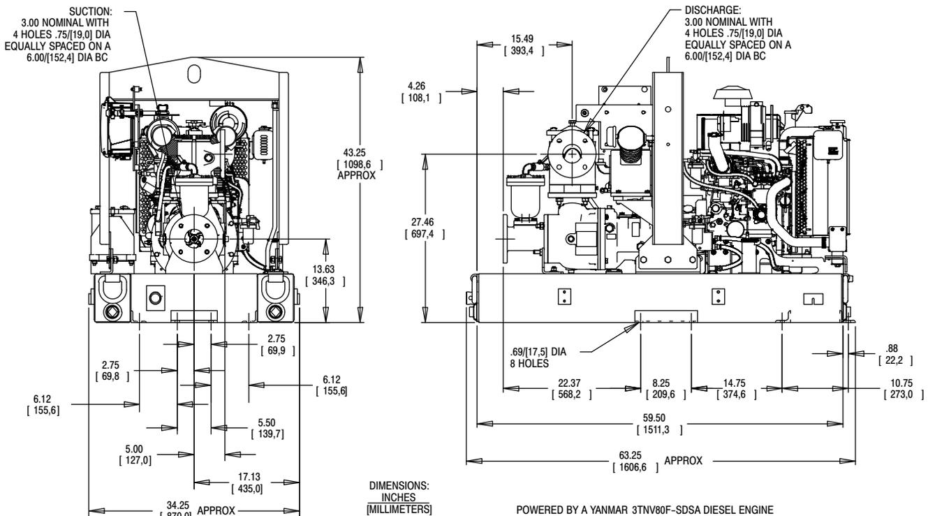
Figure 1. Pump Model PAV3B60C-3TNV80F FT4
