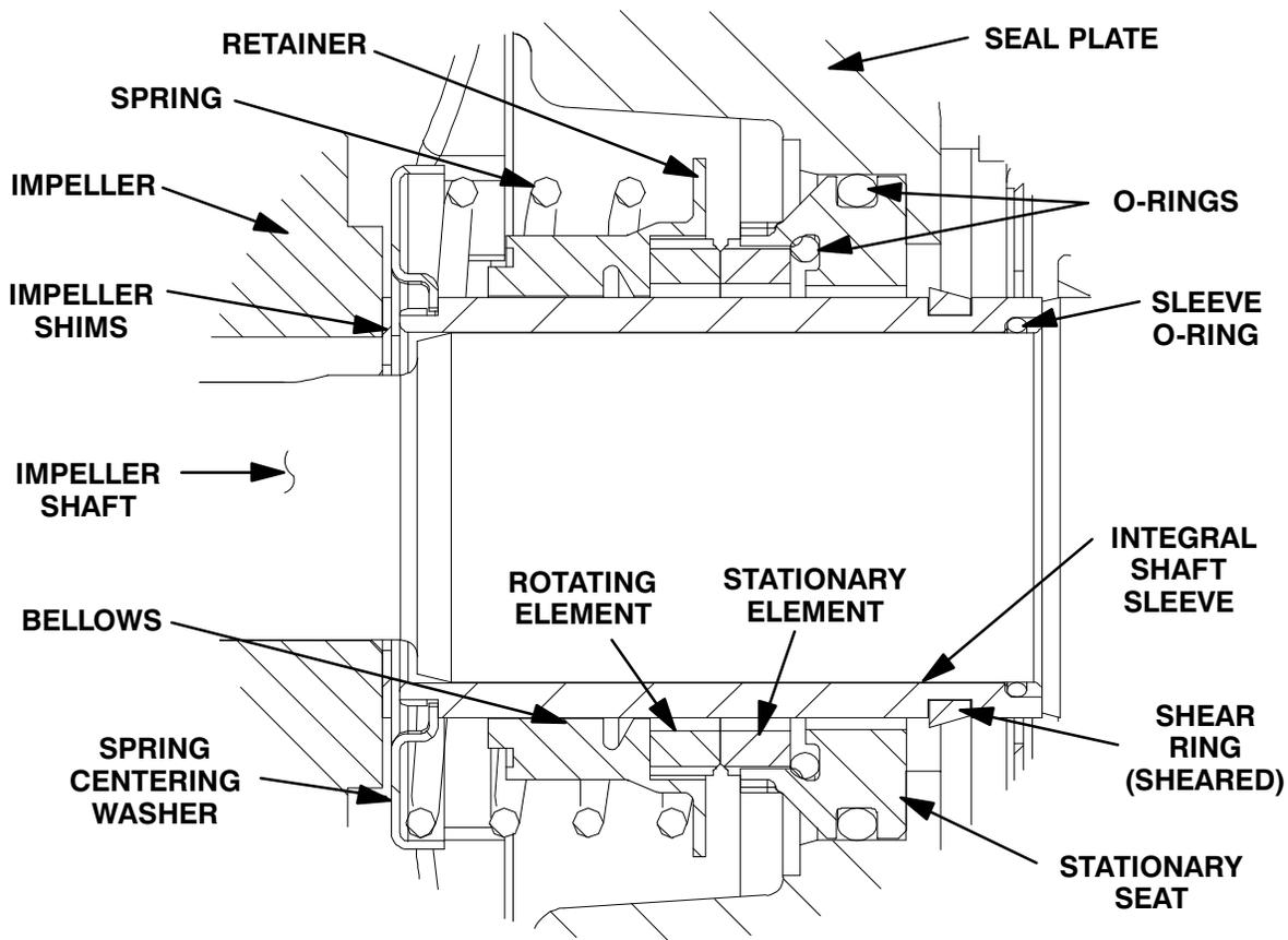
Figure 9. Seal Assembly
