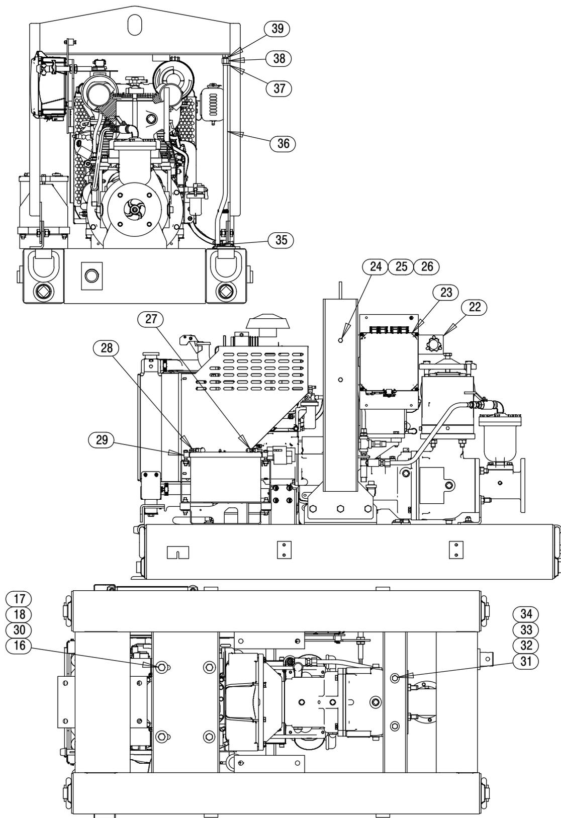
Figure 2. Pump Model PAV3B60C-3TNV80F FT4 (cont'd)
