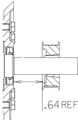
Figure 8. Drive Sprocket Positioning
