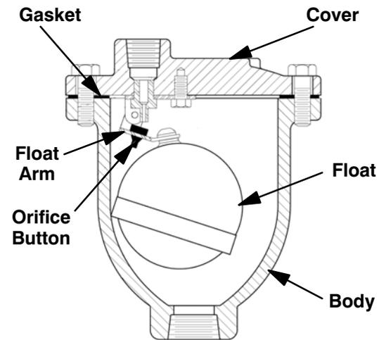
Figure 7. Priming Chamber
