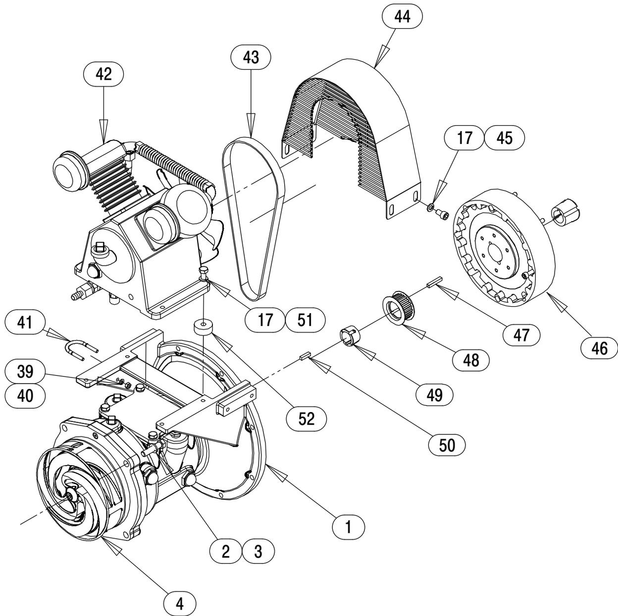
Figure 4. Pump End Assembly (cont'd)
