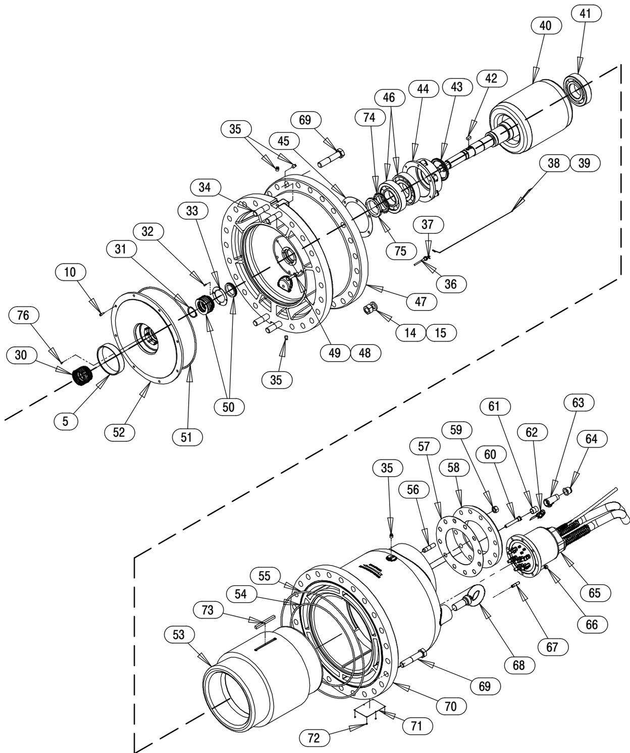
Figure E-2. S8D1-E275 460/3 & 575/3 Pump Assembly (con't)
