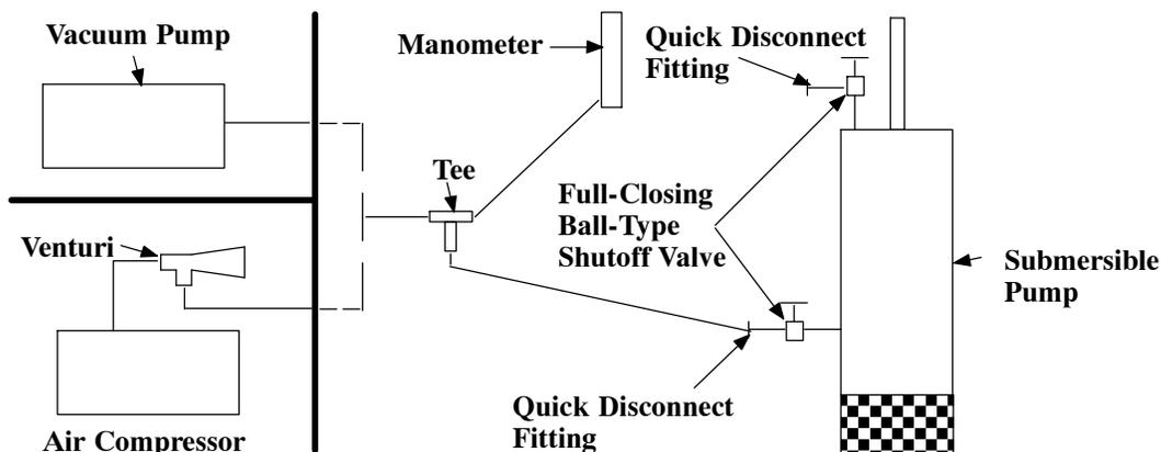
Figure E-10. Vacuum Test System
