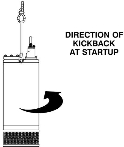
Figure C-1. Checking Pump Rotation
