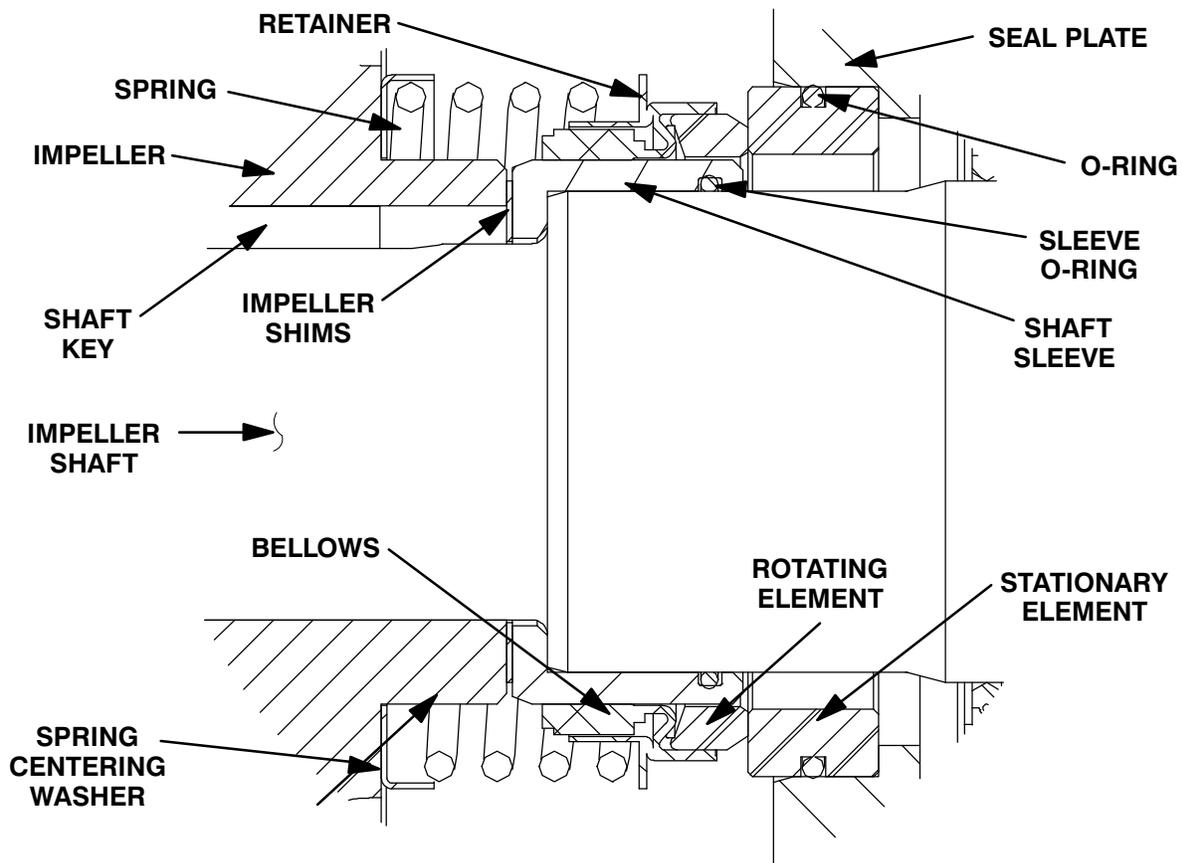
Figure 10. Seal Assembly
