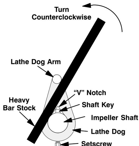
Figure 9. Loosening Impeller
