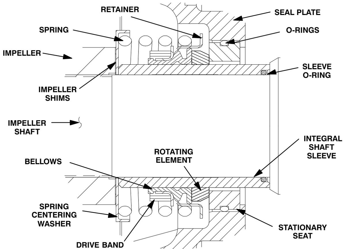
Figure 10. Seal Assembly
