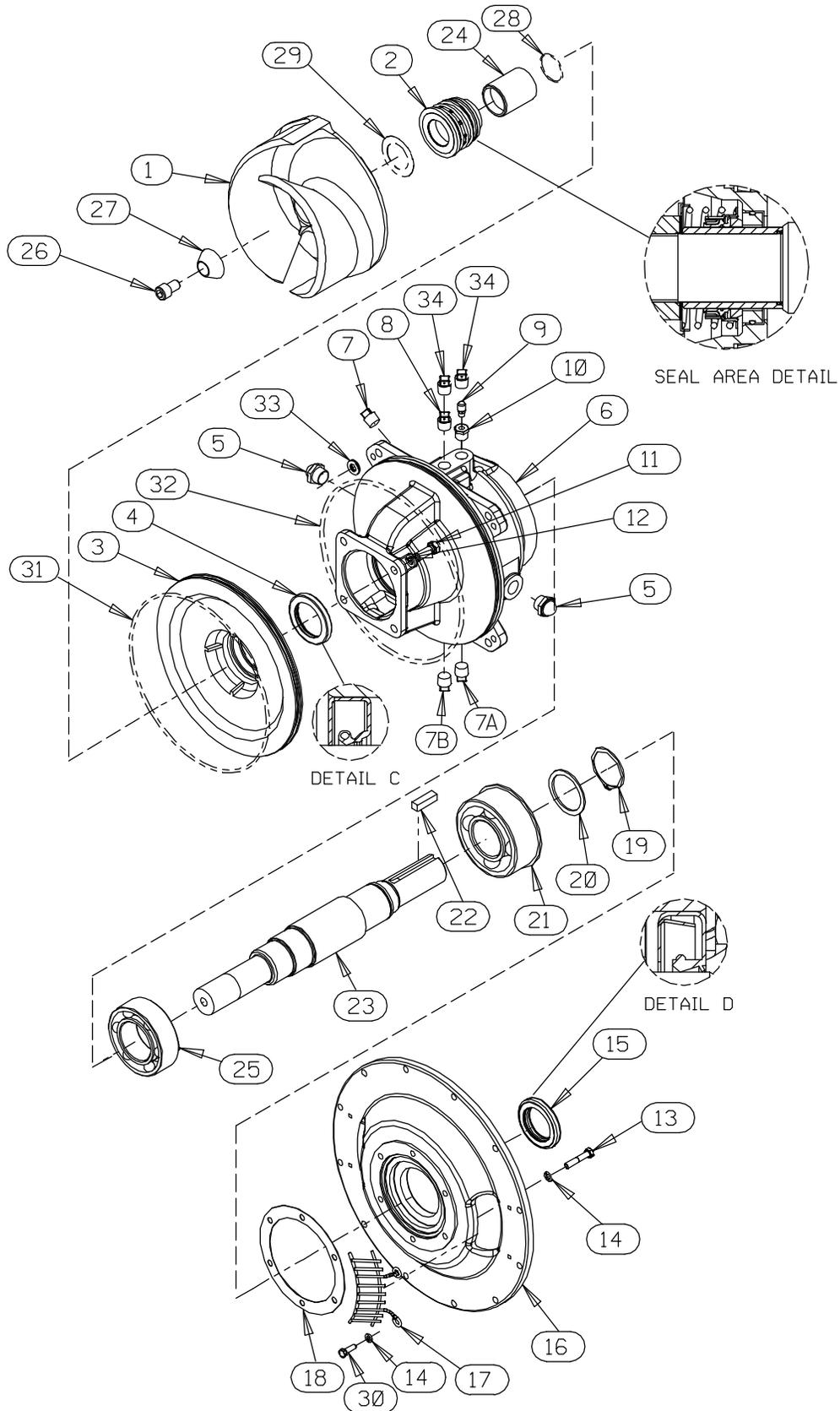
Figure 5. 44163-504 Repair Rotating Assembly
