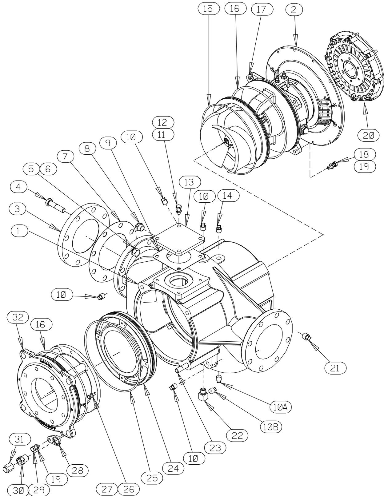
Figure 4. 66F60—(SAE 3/10) Pump End Assembly
