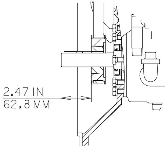
Figure 8. Drive Sprocket Positioning
