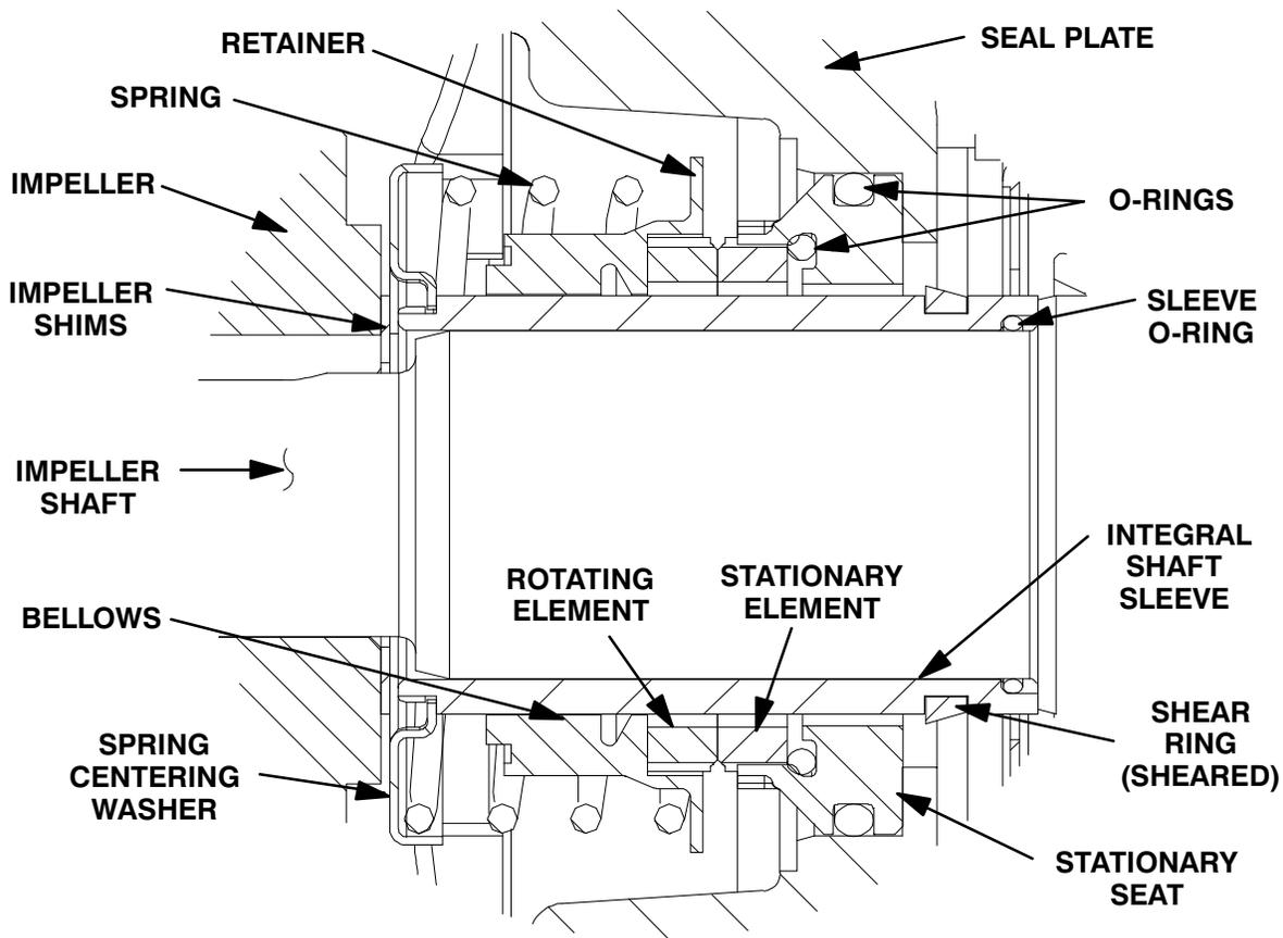
Figure 9. Cartridge Seal Assembly
