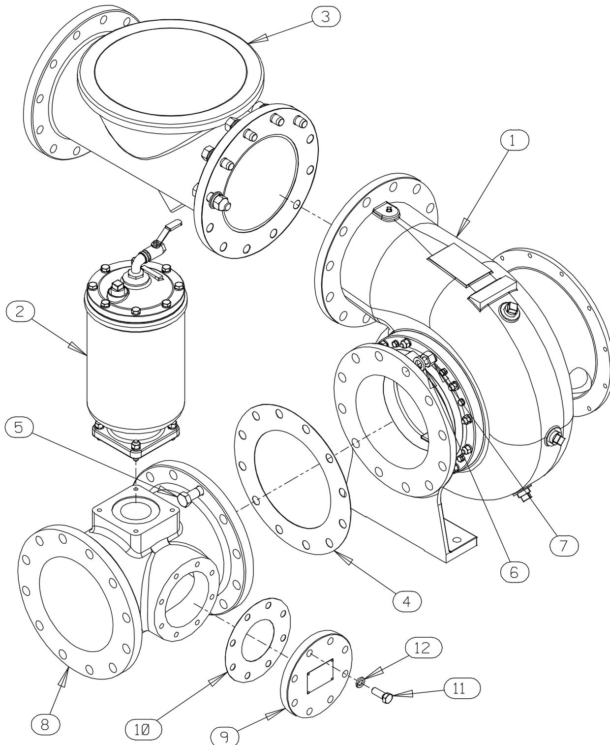
Figure 3. PA10A60—(SAE 3/11.5) Pump Assembly
