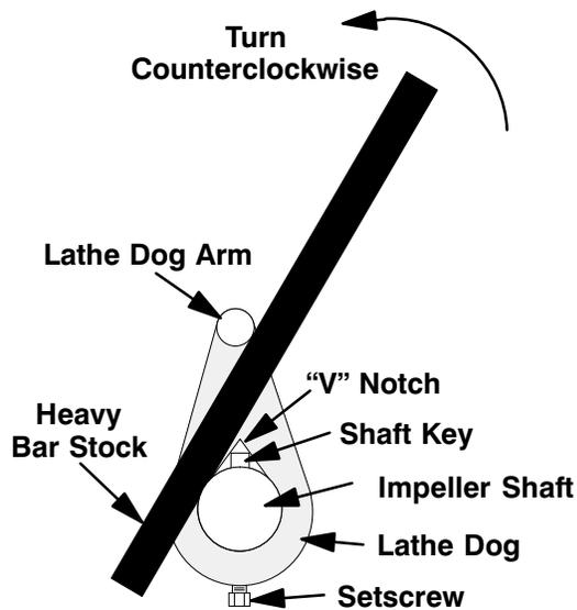
Figure 8. Loosening Impeller
