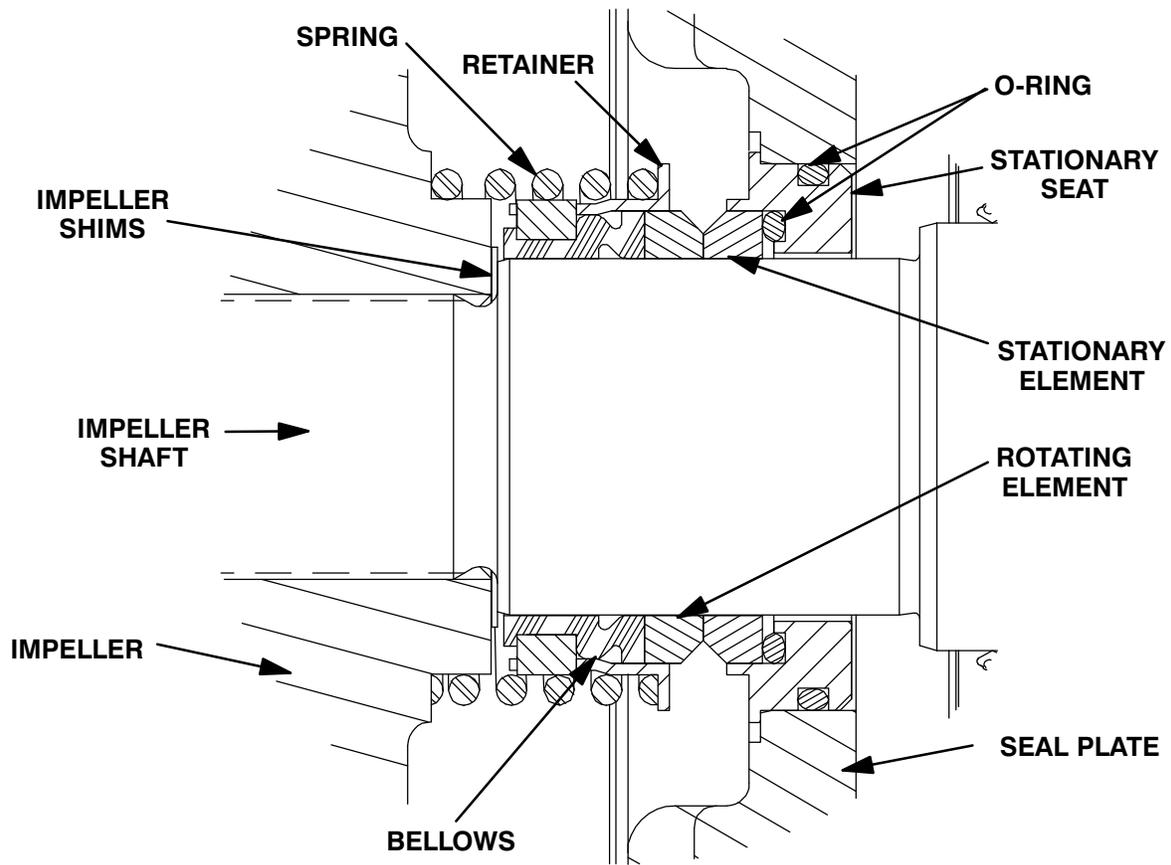
Figure 9. Seal Assembly
