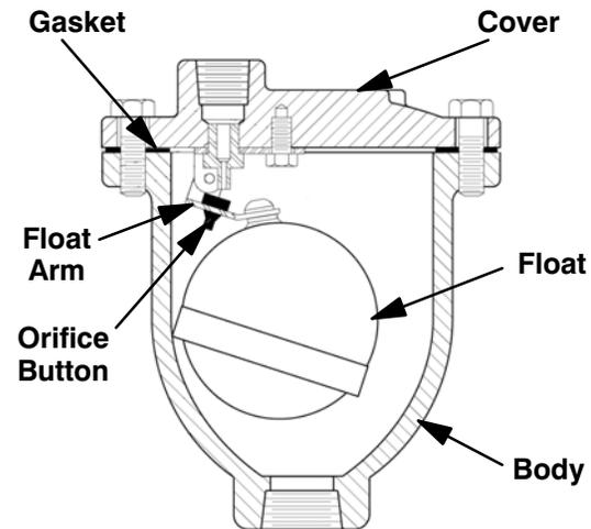
Figure 6. Priming Chamber
