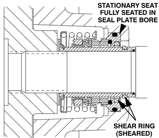
**Figure 10. Seal Fully Installed**
