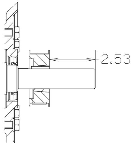
**Figure 7. Drive Sprocket Positioning**
