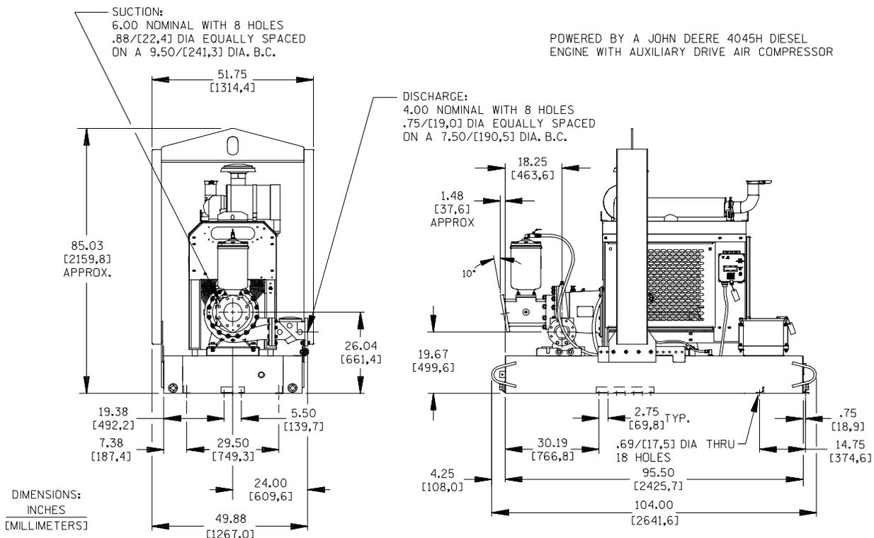
Figure 1. Pump Model PA4B60-4045H
