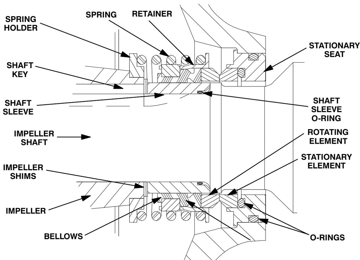
Figure 9. 46512-048 Seal Assembly
