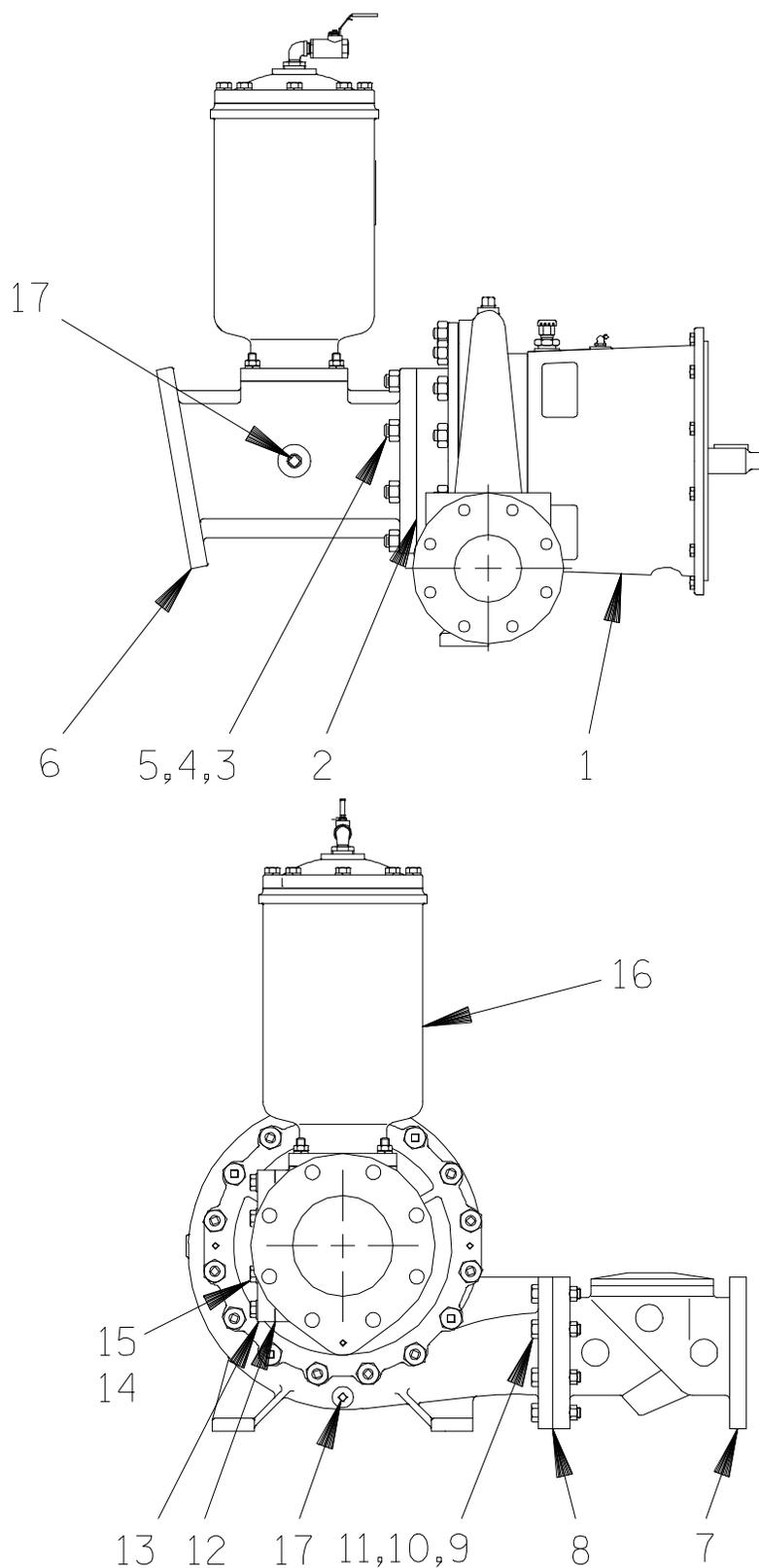
Figure 3. PA4B60-(SAE 4/10) Pump End Assembly
