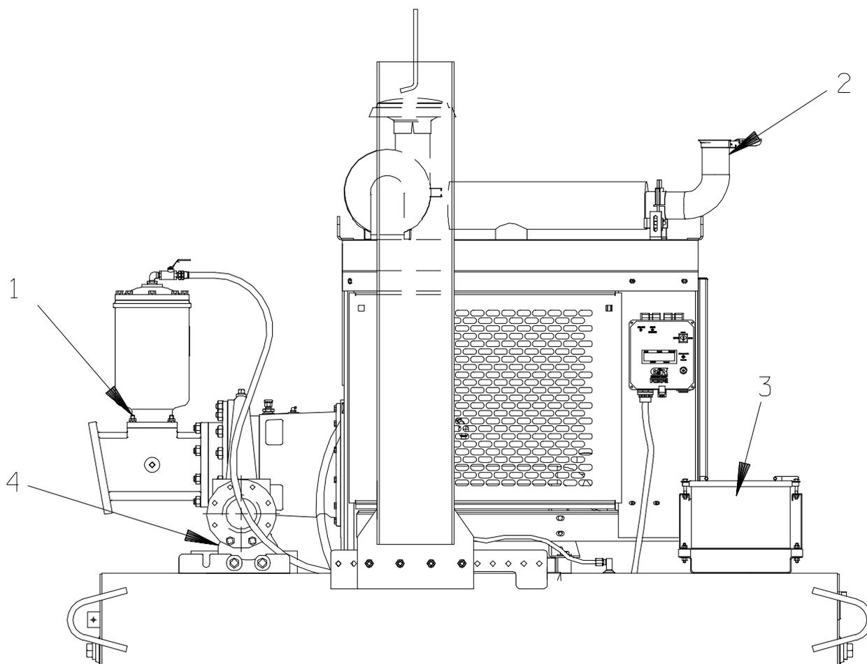
Figure 1. Pump Model PA4B60-4045H
