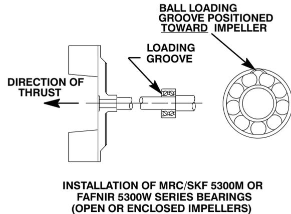
**Figure 8. Bearing Installation**
