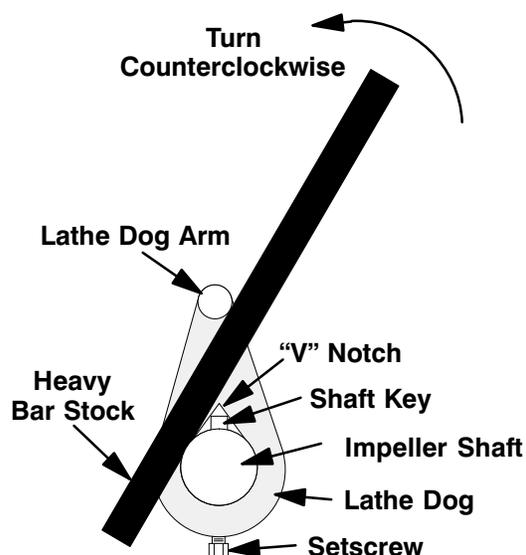
Figure 9. Loosening Impeller
