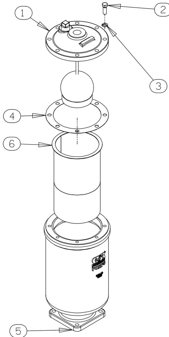
Figure 7. 46112-709 Priming Chamber Assembly
