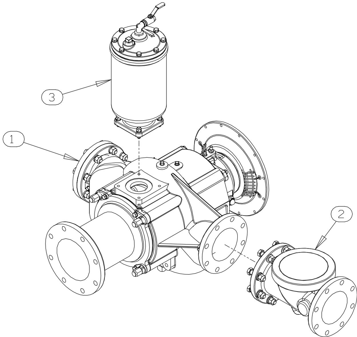
Figure 3. PA6C60-(4045H) Pump Assembly
