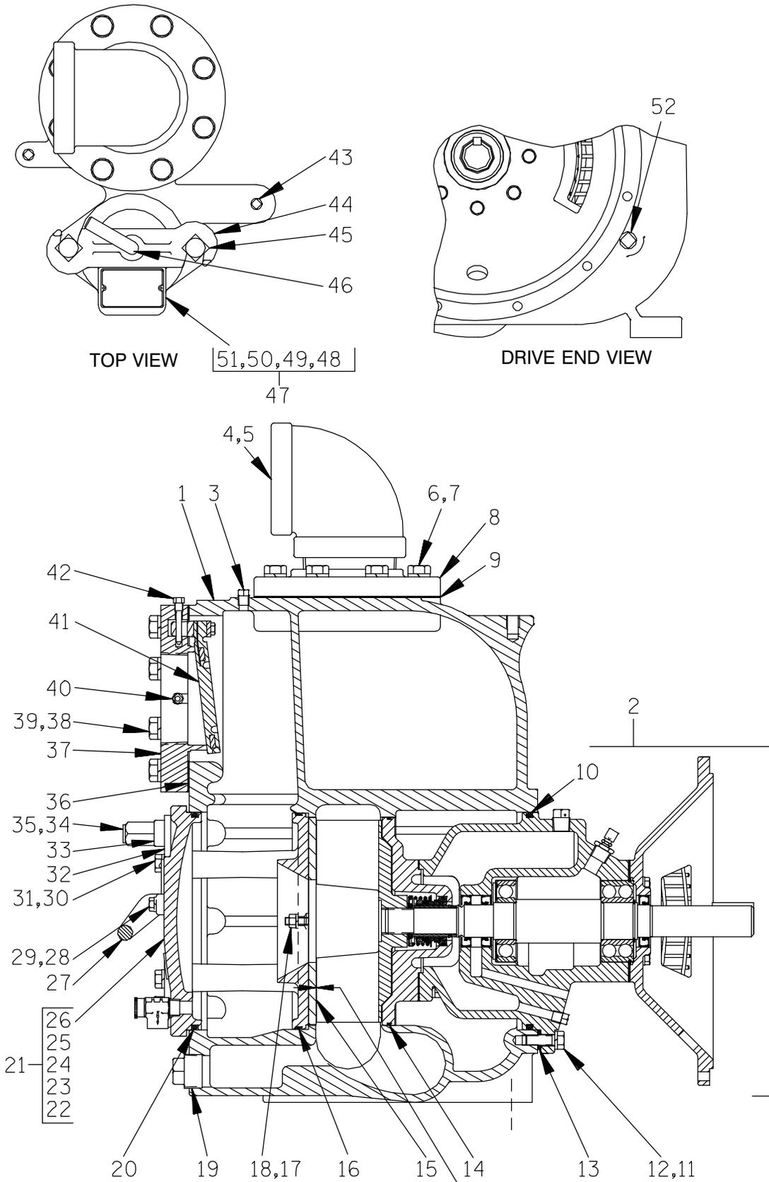
Figure 3. T4A60S-(SAE 4/10) Pump End Assembly
