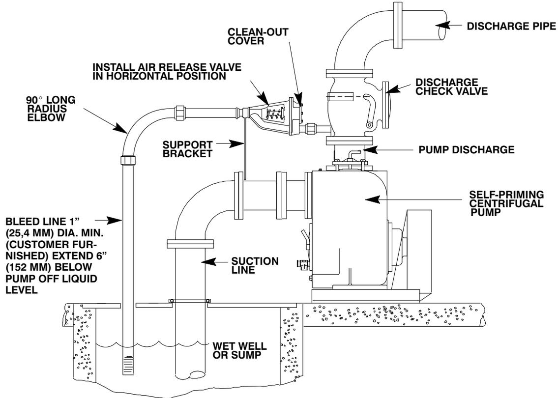
**Figure 5. Typical Automatic Air Release Valve Installation**
