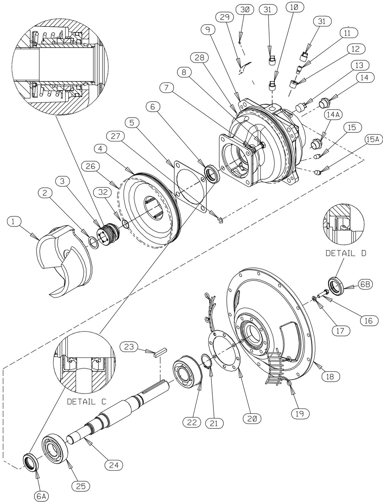
Figure 4. 44163-347 Repair Rotating Assembly
