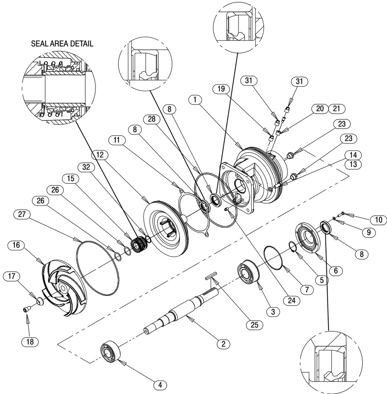
Figure 2. Repair Rotating Assemblies
