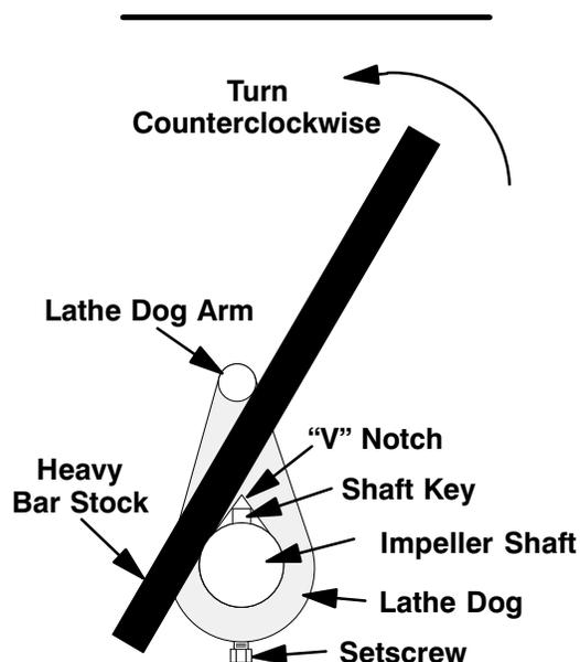
Figure 3. Loosening Impeller
