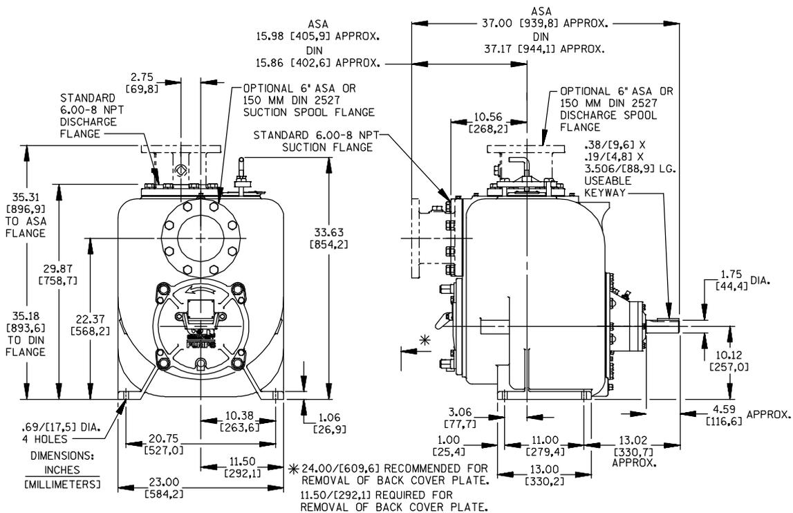
Figure 1. Pump Model U6B60S-B Including /F, /FM, /WW
