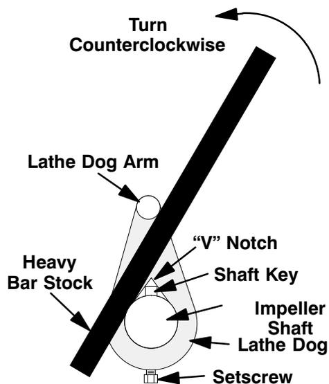
Figure 5. Loosening Impeller
