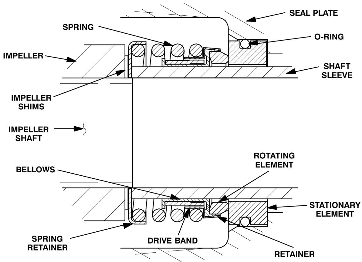
Figure 6. Seal Assembly
