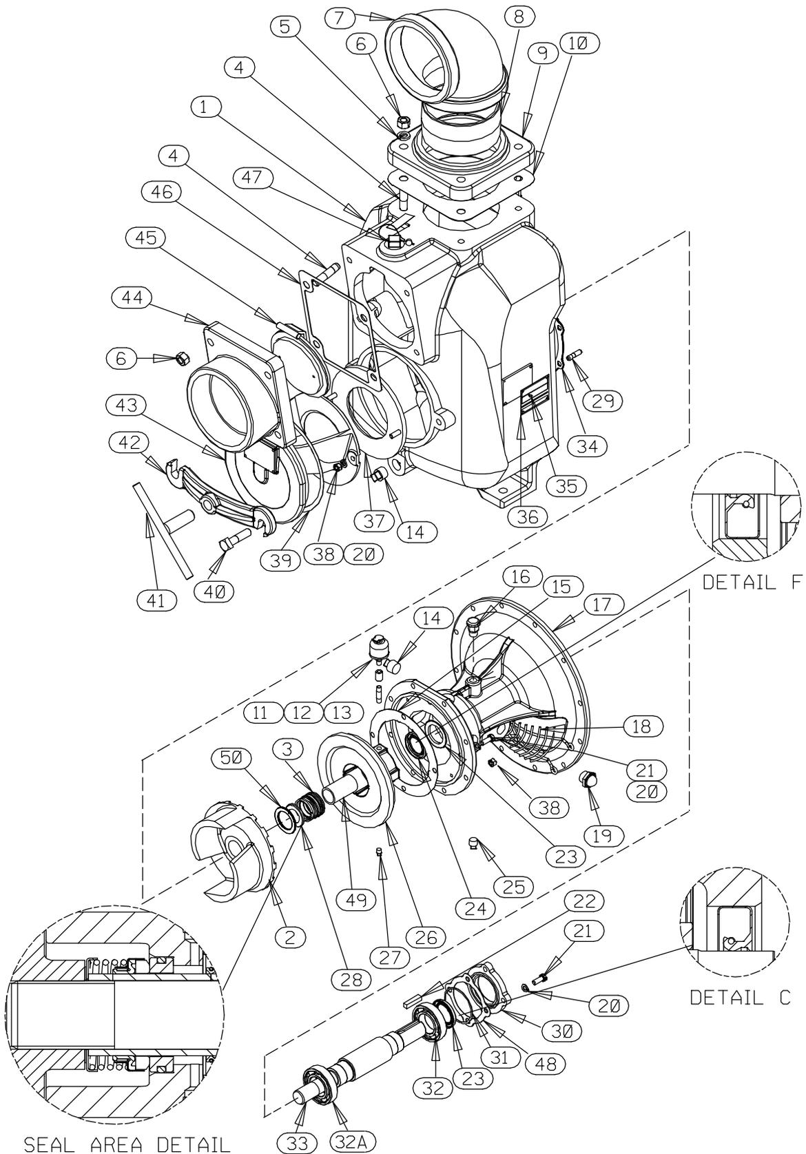
Figure 3. 16D60-(SAE 4/10) Pump End Assembly
