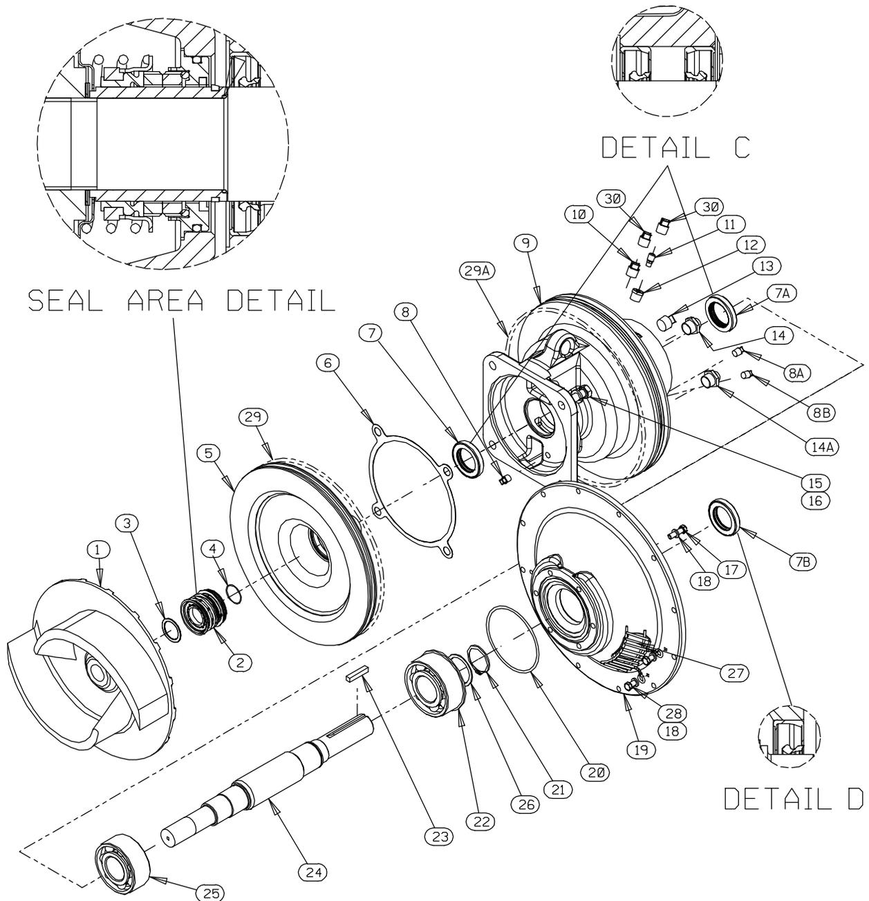
Figure 4. Repair Rotating Assembly
