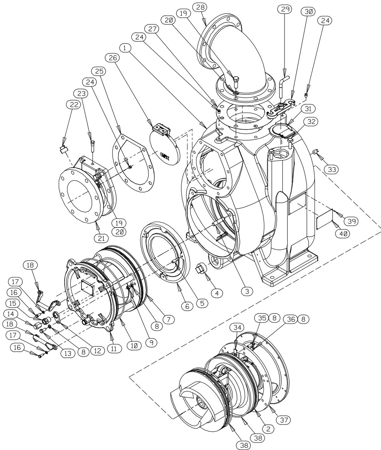
Figure 3. T8A60S-(SAE 3/10) Pump End Assembly
