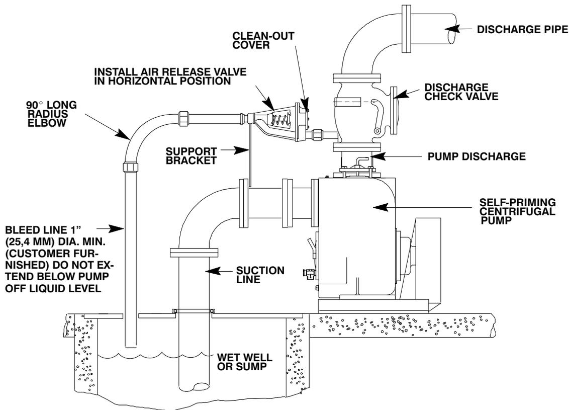
**Figure 7. Typical Automatic Air Release Valve Installation**
