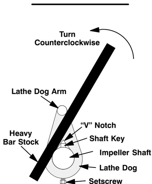
**Figure 6. Loosening Impeller**
