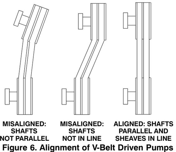
**MISALIGNED: SHAFTS NOT PARALLEL    MISALIGNED: SHAFTS NOT IN LINE    ALIGNED: SHAFTS PARALLEL AND SHEAVES IN LINE**
