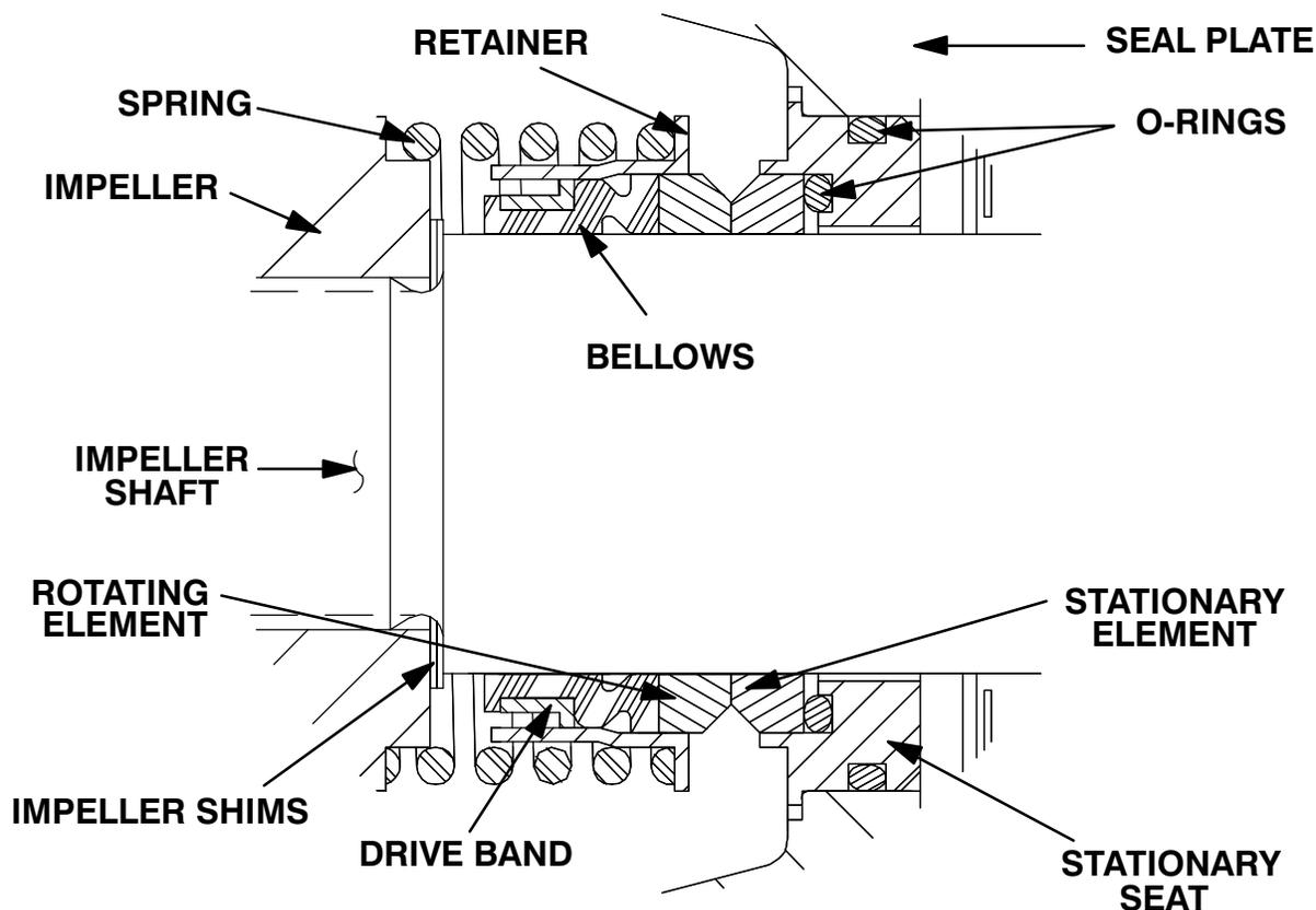
Figure 6. Seal Assembly
