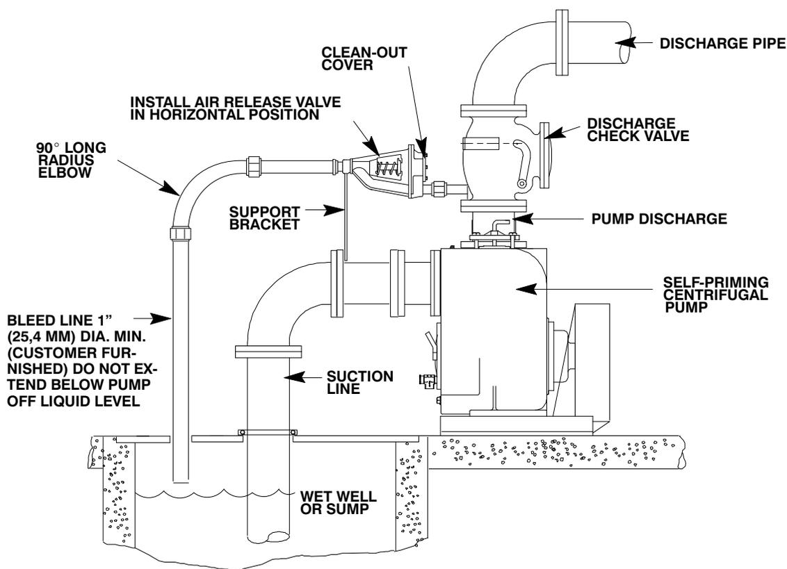
**Figure 3. Typical Automatic Air Release Valve Installation**
