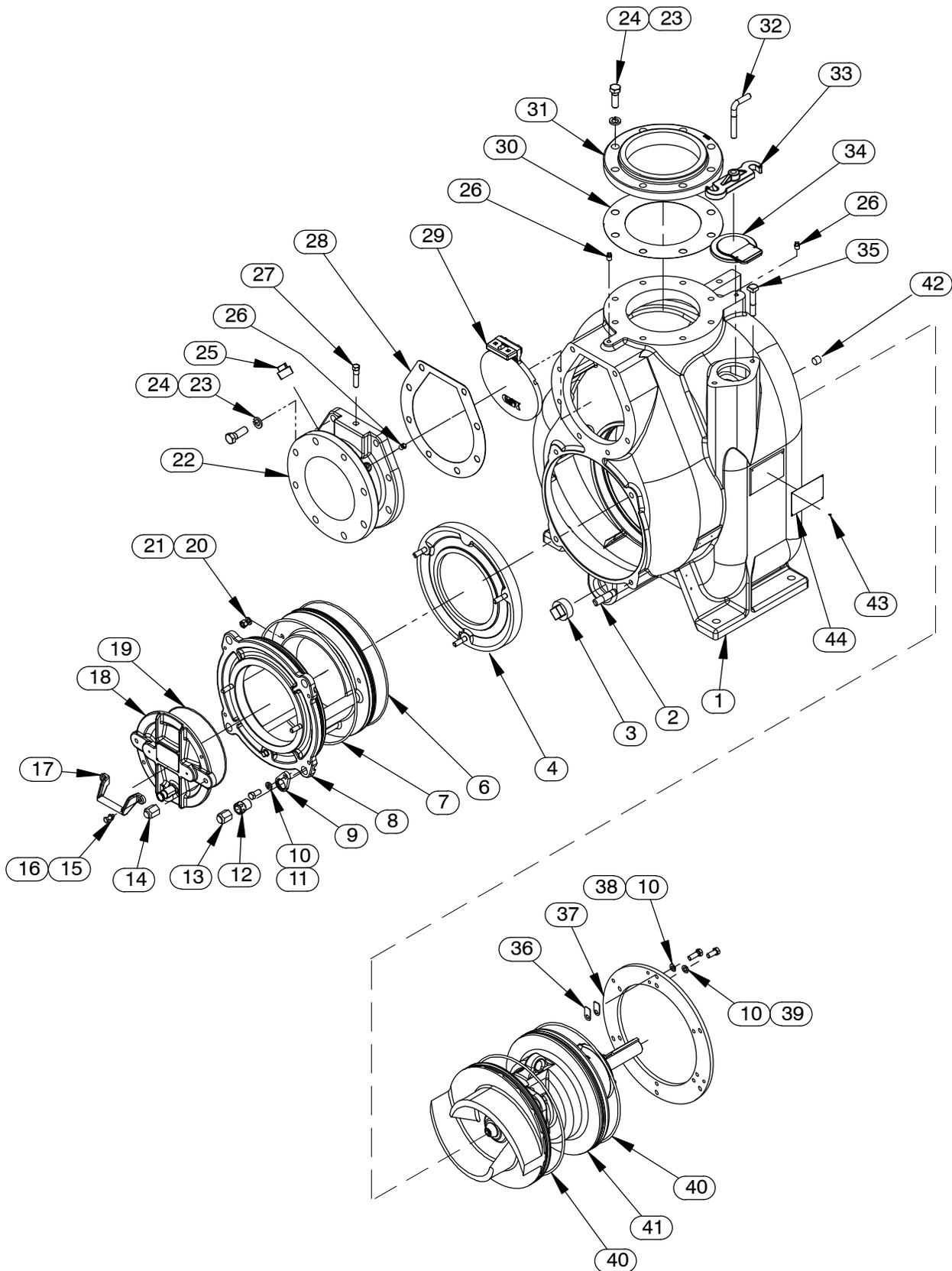
Figure 1. Pump Model T8A61S-B, including /F, /FM
