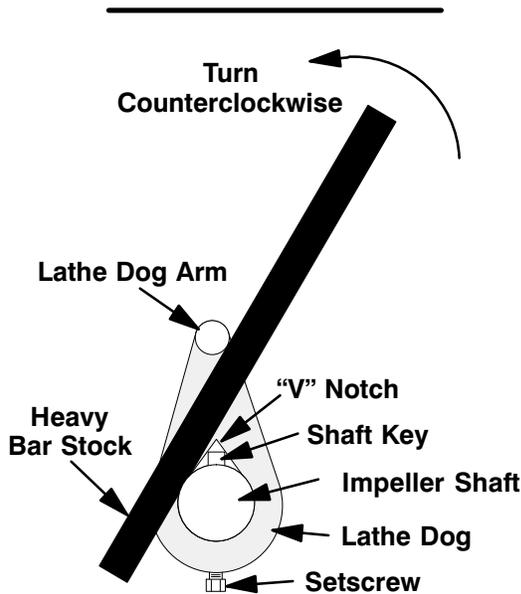
**Figure 3. Loosening Impeller**
