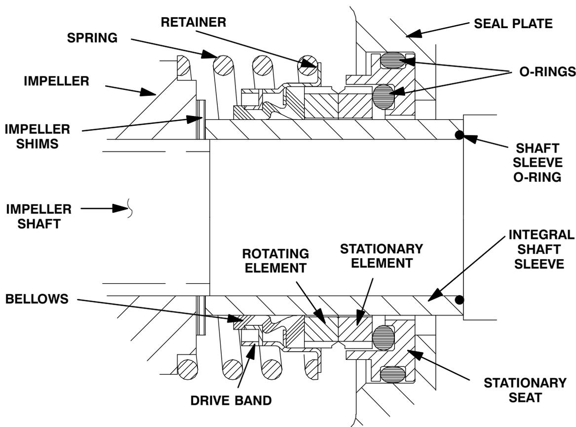
Figure 4. Seal Assembly
