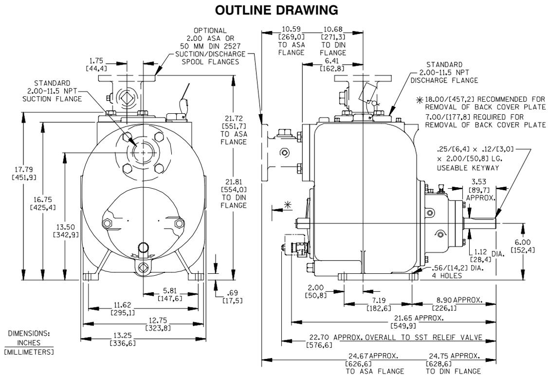
**Figure 1. Pump Model T2A71–B, Including /F, /FM**
