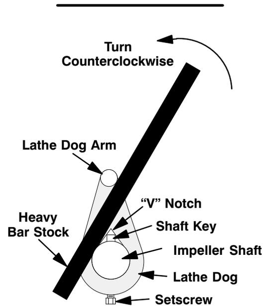
Figure 3. Loosening Impeller
