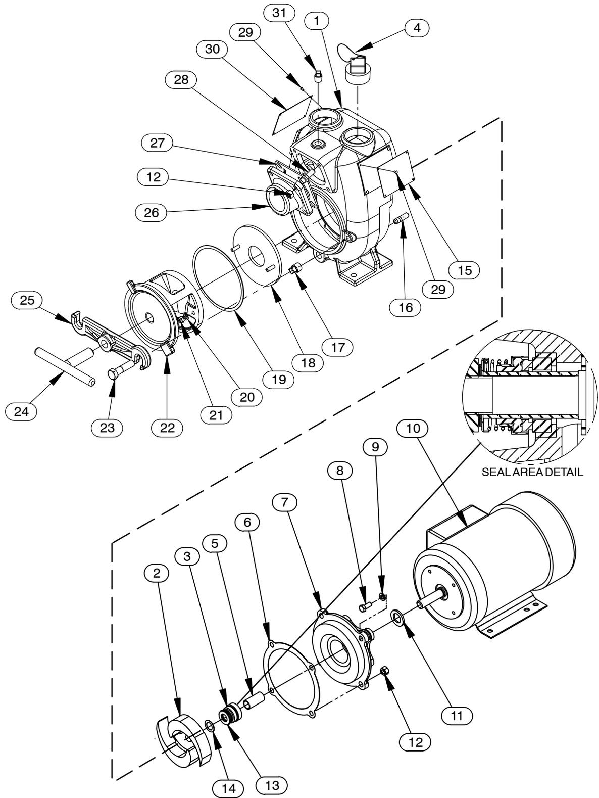
Figure 1. Pump Models 11 1/2A3-KW1.5 3P
