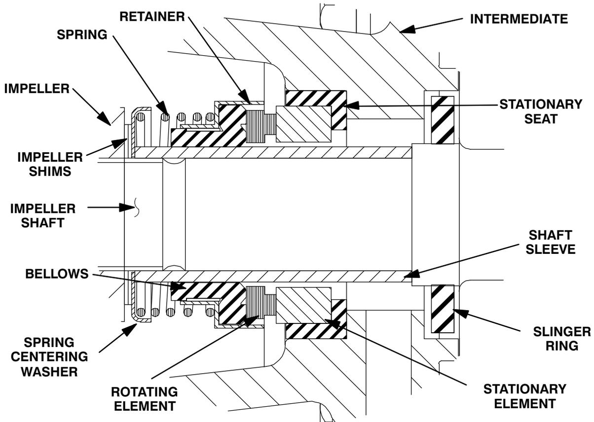
Figure 2. Seal Assembly
