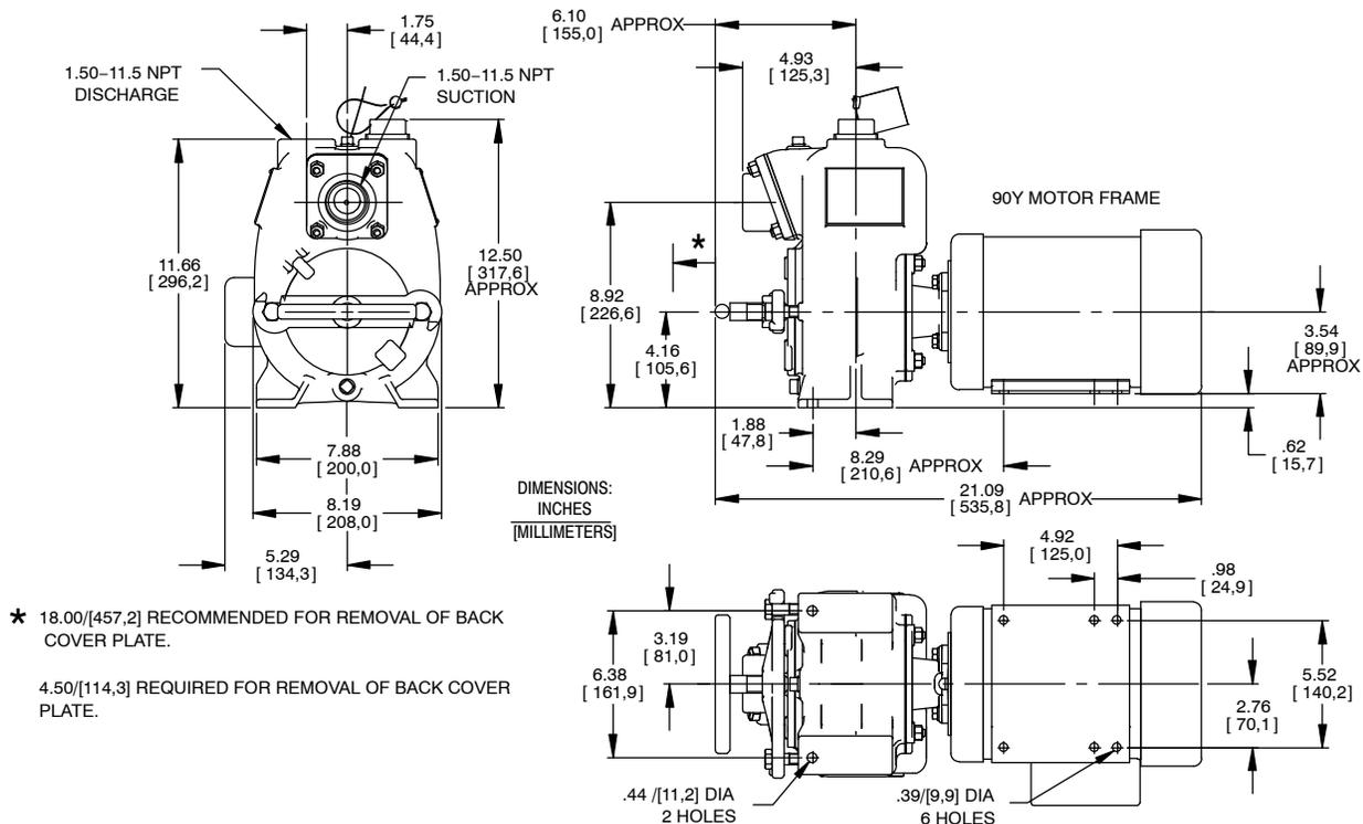
**Figure 1. Pump Models 11 1/2A3-KW1.5 3P**
