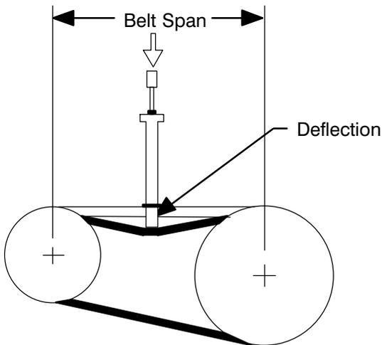
**Figure B-6. Belt Tension Measurement**
