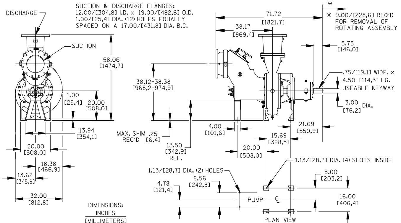
Figure B-1. Pump Model 112G60-B
