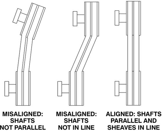
**MISALIGNED: SHAFTS NOT PARALLEL**      **MISALIGNED: SHAFTS NOT IN LINE**      **ALIGNED: SHAFTS PARALLEL AND SHEAVES IN LINE**
