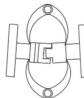
**Figure B-3. Aligning Spider-Type Couplings**
