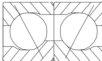
**Figure E-2. Correct Bearing Mounting**
