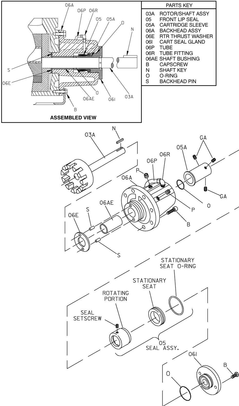
Figure F-2. Option 60N Positive Drive Seal
