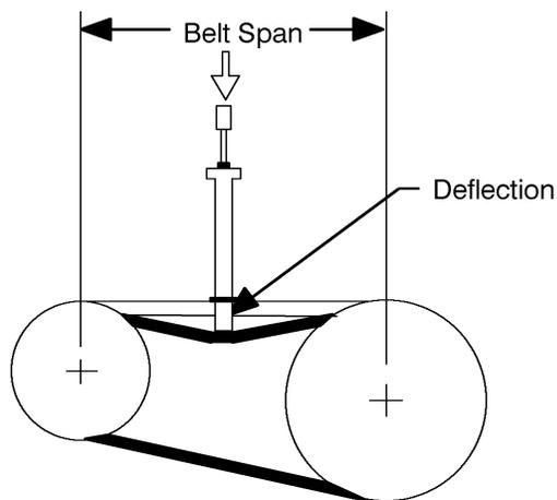
Figure B-5. Belt Tension Measurement
