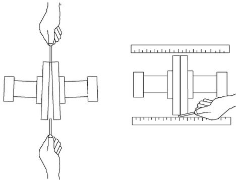
**Figure B-3. Aligning Non-Spider Type Coupling**
