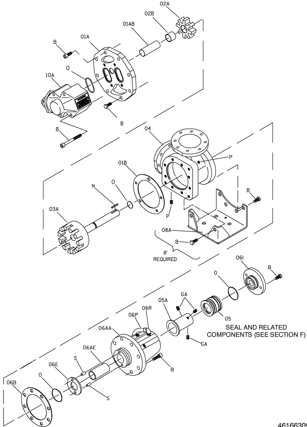
Shown: Standard S Size Model With 90° Ports, Removeable Foot Bracket, Backhead Cooling Jacket And Head-Mounted Relief Valve. Cast Foot Bracket Standard on T Size Models. All Models Available With Head Jacket. Cover-plate Kit Replaces Relief Valve When Not Used.
