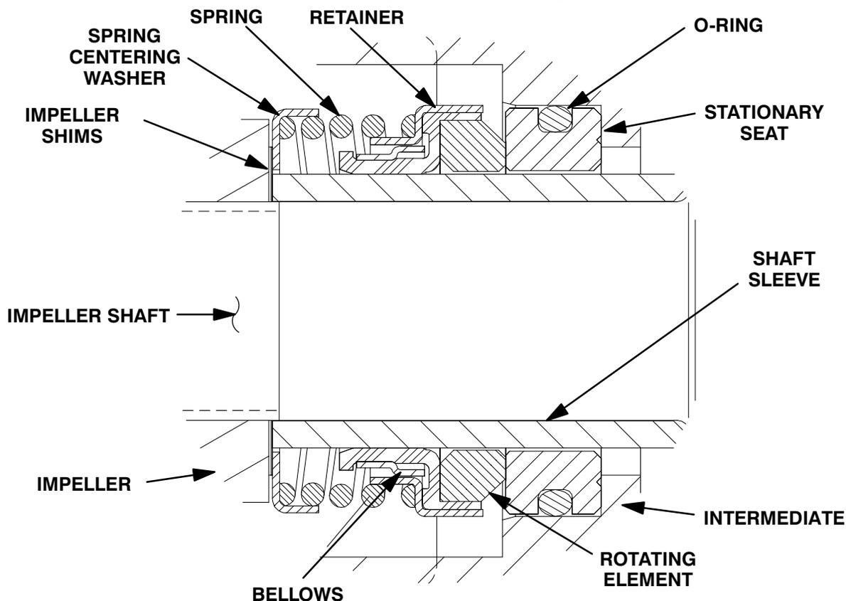
Figure 4. 25285-855 Seal Assembly
