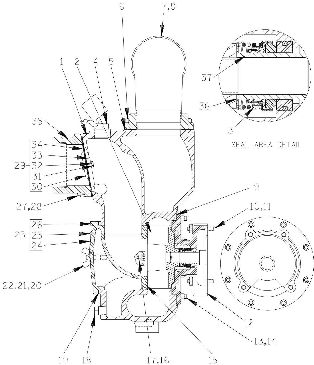
Figure 3. Pump End Assembly 14D52-(CH13) PPO
