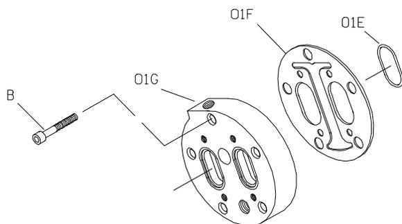
Figure E-2. Typical Head Jacket Assembly
