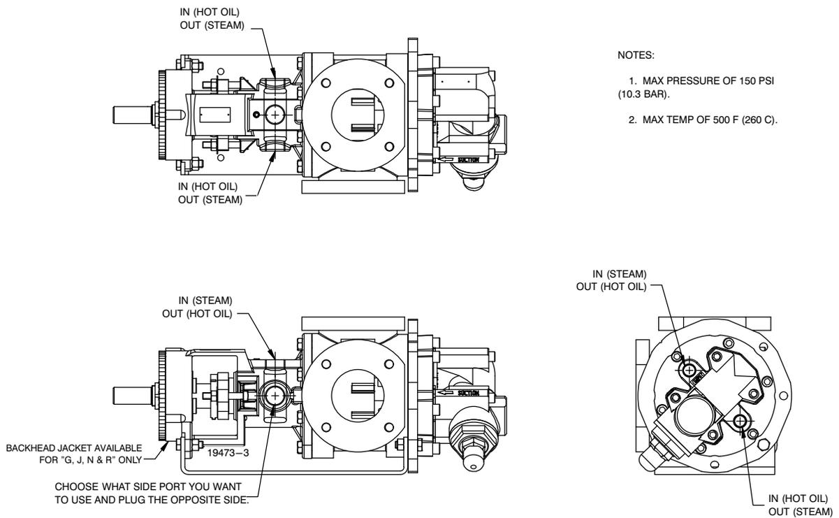
Figure H-1. Inlet / Outlet Location
