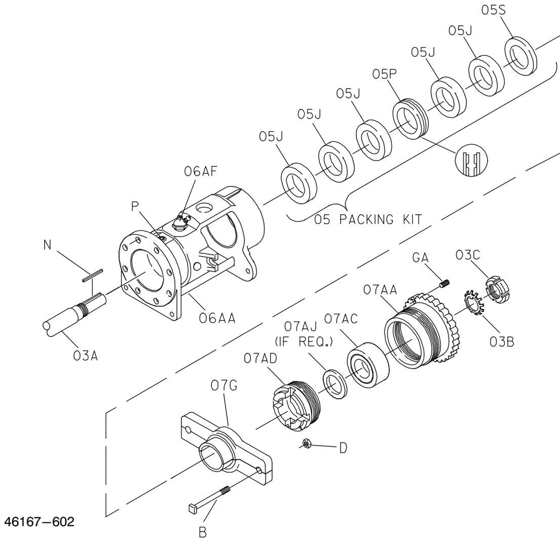
Figure F-4. Standard Packing Seal (Option 65)
