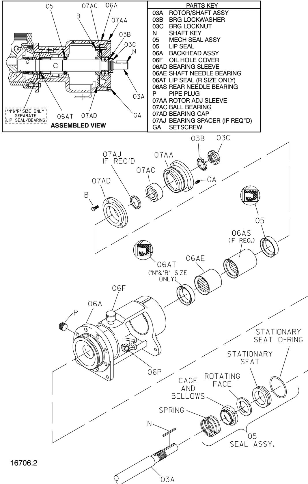
Figure F-1. Standard Friction Drive Mechanical Seal (Option 62)
