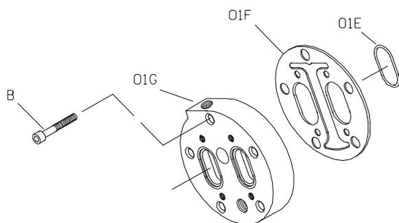
Figure E-2. Typical Head Jacket Assembly
