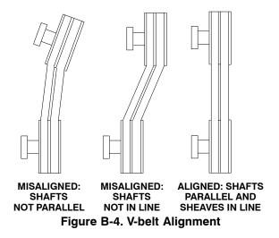
Tighten the belts in accordance with the belt manufacturer's instructions. If the belts are too loose they will slip; if they are too tight, there will be excessive power loss and possible bearing failure.
