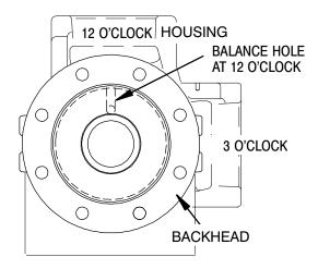
Figure E-5. Housing/Backhead Alignment
