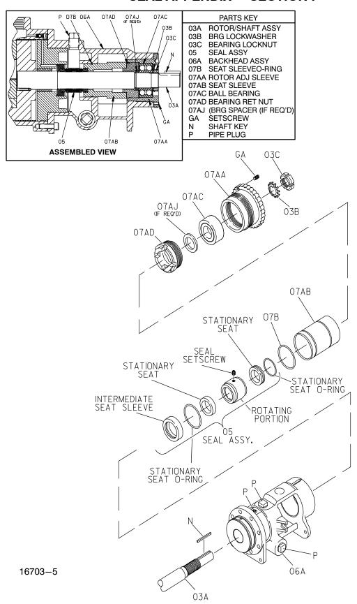
Figure F-3. Double Positive Drive (Option 60J) Seal
