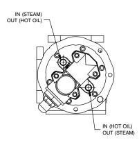
Figure H-1. Inlet / Outlet Location
