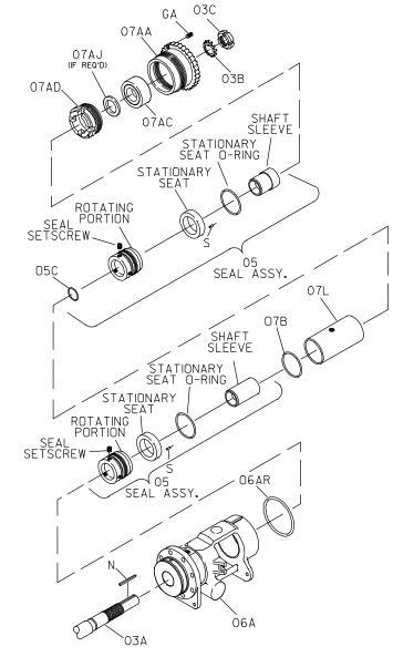
Figure F-7. Option 60S Positive Locking Tandem Mechanical Seal ("D" Size Only)
