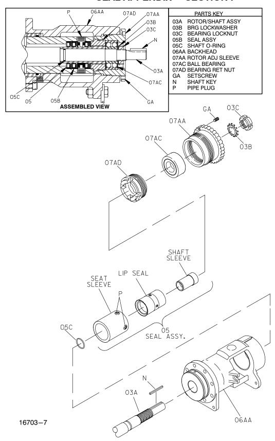
Figure F-6. Option 65E Cartridge Lip Seal ("D" Size Only)
