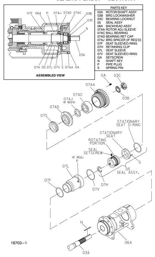
Figure F-1. Standard 60 Seal Assembly
