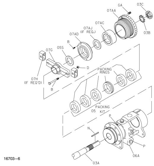
Figure F-4. Optional Packing Seal
