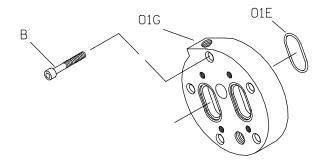
Figure E-2. Typical Head Jacket Assembly
