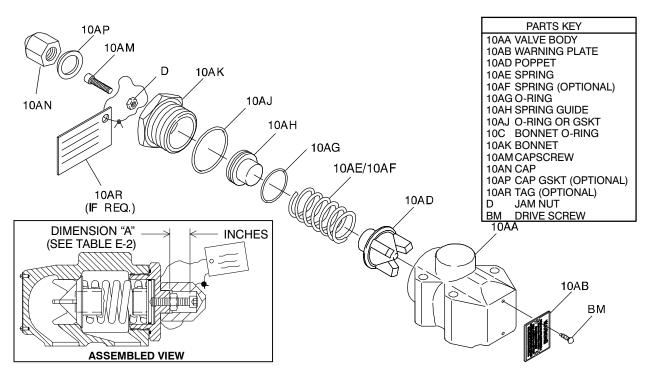
Figure E-7. Pressure Relief Valve Assembly
