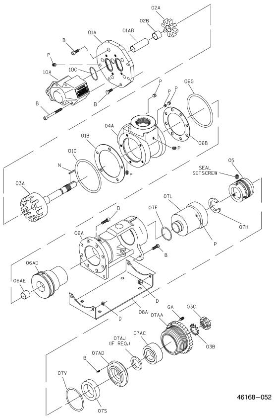
**Shown:** Standard Model With 90 Ports, Head-Mounted Relief Valve and Optional Foot Bracket. Also Available With 180 Ports And/Or Housing-Mounted Relief Valve. A Coverplate Kit Replaces Either Relief Valve When Not Used. **NOTE:** Refer to **Seal Appendix, Section F** for details of the seal assembly and related components.
