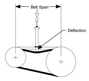
Figure B-5. Belt Tension Measurement
