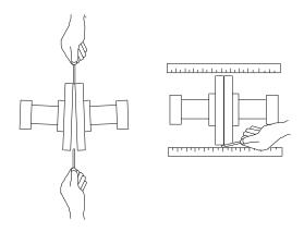
Figure B-3. Aligning Non-Spider Type Coupling
