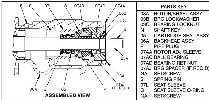
SHOWN: METAL BELLOWS TYPE SEAL. INDIVIDUAL CARTRIDGE SEAL COMPONENTS MAY VARY IN DESIGN.
