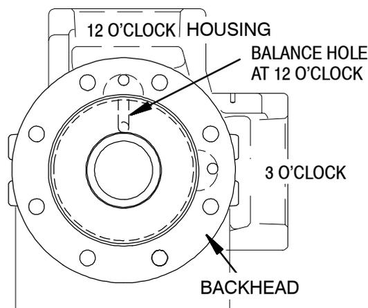
**Figure E-5. Housing/Backhead Alignment**
