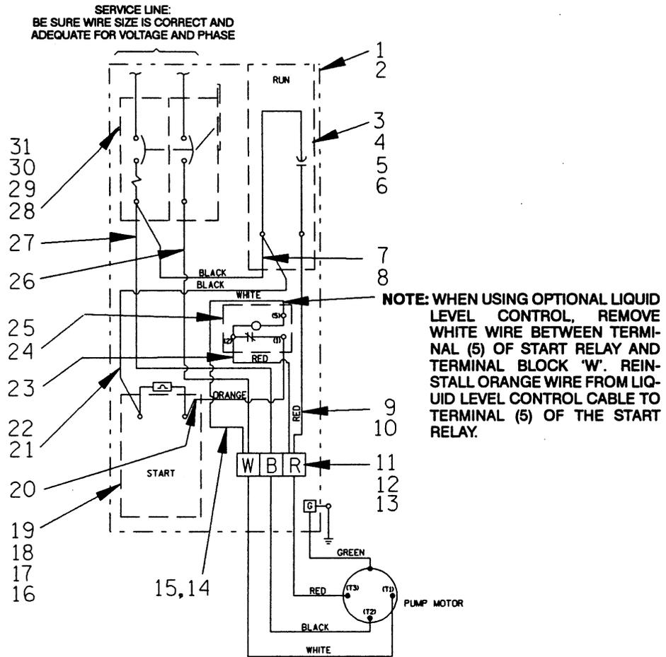
Figure 7. Pictorial Diagram - 47631-068 (115V 1P) And 47631-069 (230V 1P) Control Boxes
