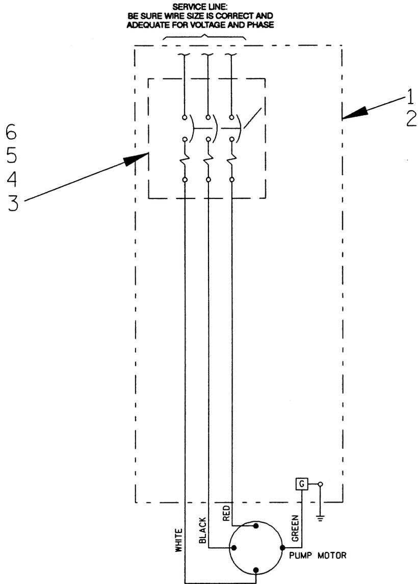
Figure 8. Pictorial Diagram - 47631-067 (230V 3P) Control Box
