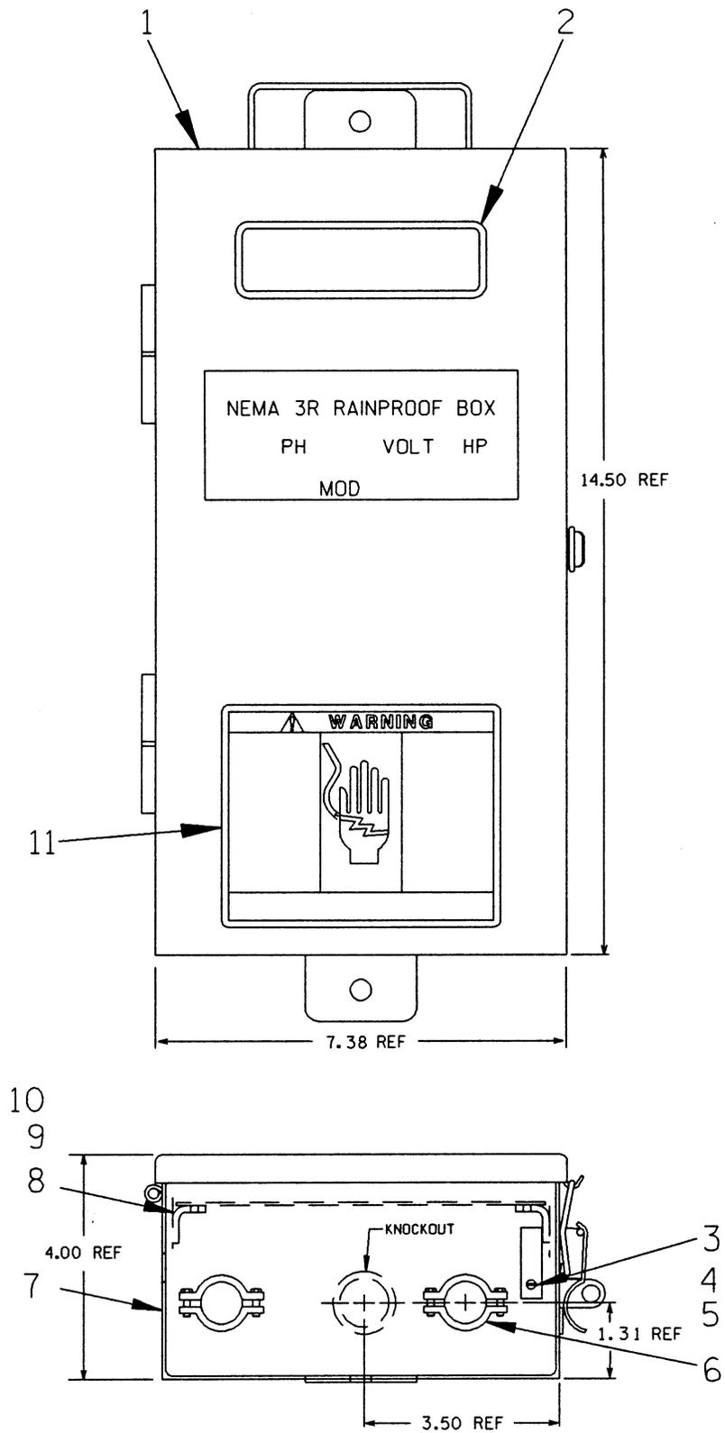
Figure 3. Control Box Dimensions
