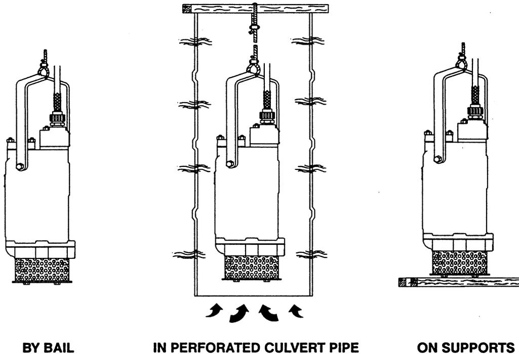
Figure 2. Typical Pump Installations
