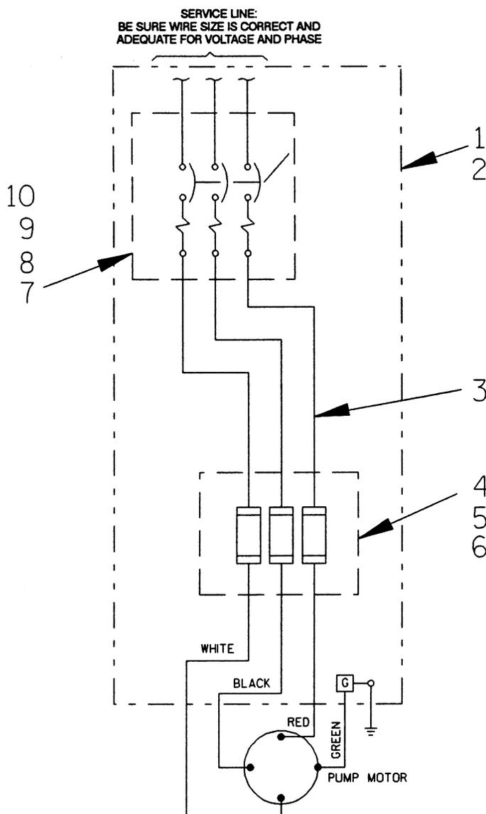
Figure 9. Pictorial Diagram - 47631-066 (460V 3P) and 47631-078 (575V 3P) Control Boxes
