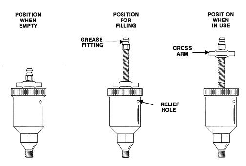
Figure 4. Automatic Lubricating Grease Cup
