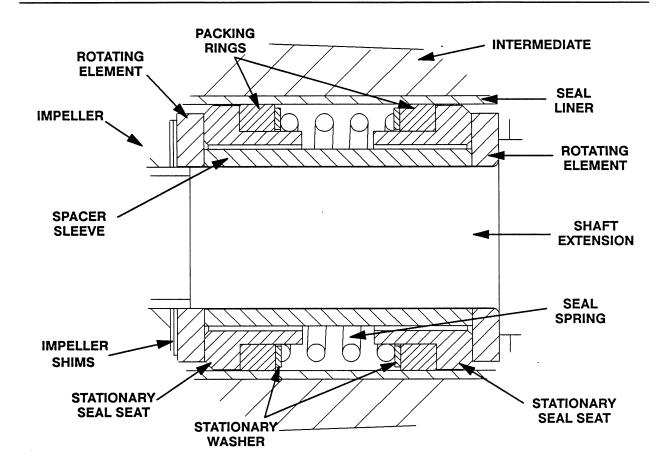
Figure 4. 46521-013 Seal Assembly
