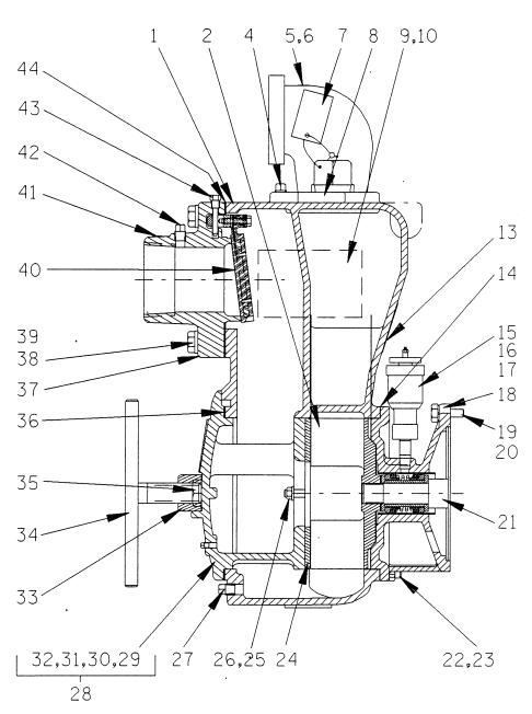
Figure 2. Pump End 13C2-(M20 S/G)
