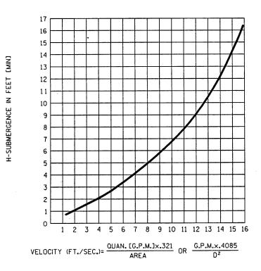
Figure 3. Recommended Minimum Suction Line Submergence vs. Velocity
