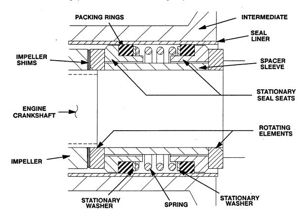
Figure 4. GS1000-C Seal Assembly
