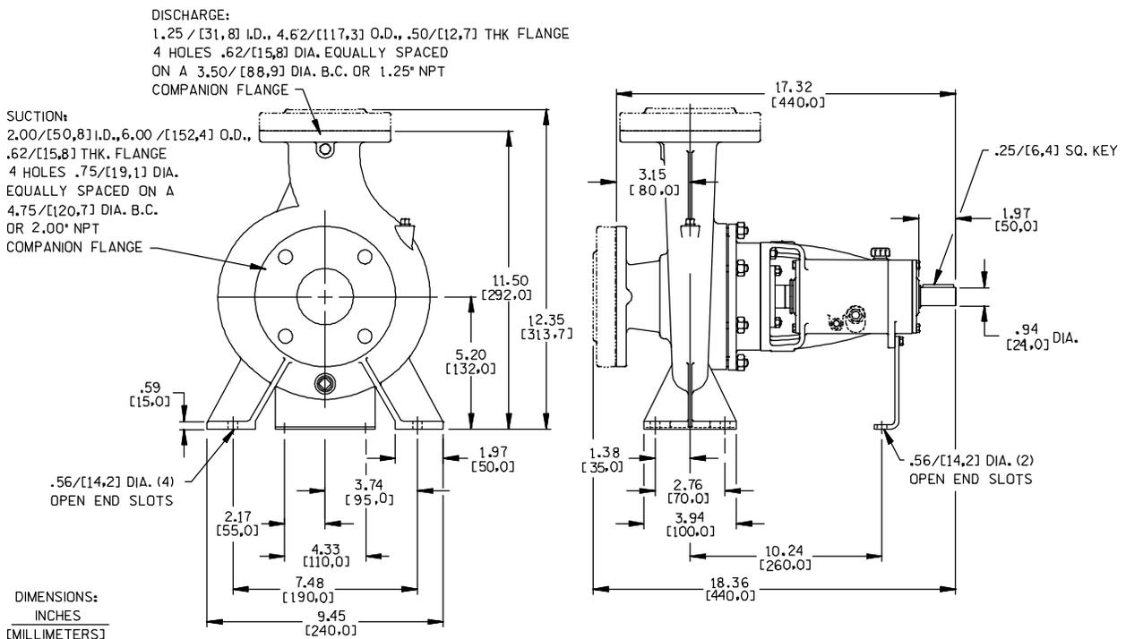
**Figure 1. Pump Model VG1 1/4B3-B**
