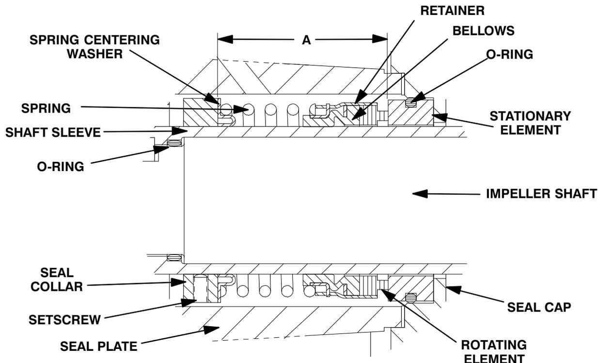
**Figure 2. 25271-032 Seal Assembly**
