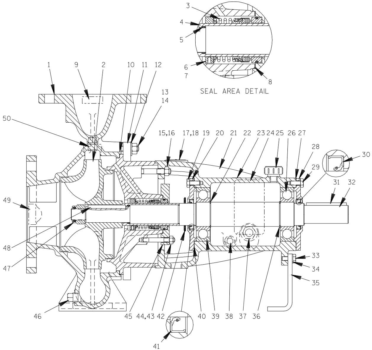
Figure 1. Pump Model VG1 1/4B3-B
