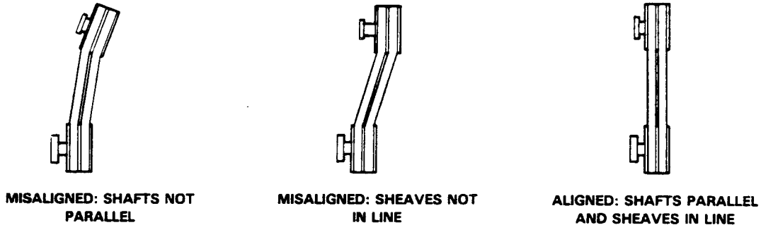
Figure 3C. Alignment of V-Belt Driven Pumps
