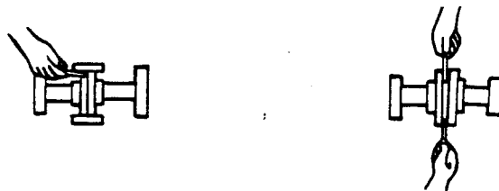
Figure 2B. Aligning Non-Spider Type Couplings
