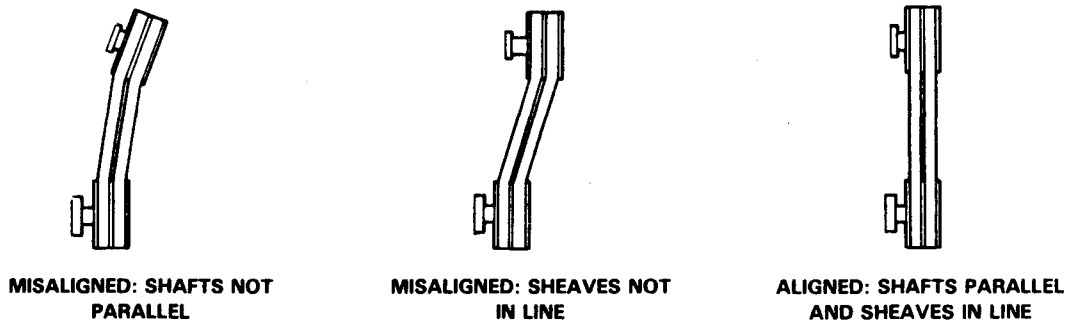
Figure 3C. Alignment of V-Belt Driven Pumps
