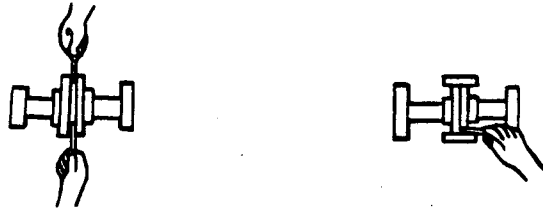
Figure 3B. Aligning Non-Spider Type Couplings
