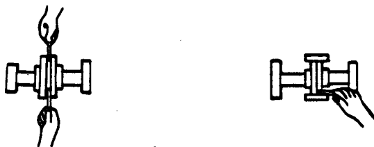
Figure 3B. Aligning Non-Spider Type Couplings
