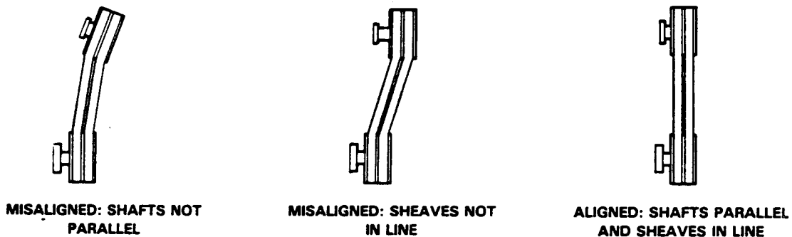
Figure 3C. Alignment of V-Belt Driven Pumps
