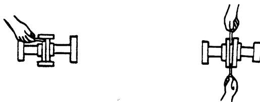
Figure 2B. Aligning Non-Spider Type Couplings
