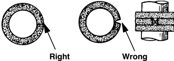
**Step 2:** It is critical that the ends of the cut packing rings meet in a tight parallel fit to ensure proper sealing. Check this fit; it should be correct if the packing was cut while wrapped around a rod, but if the packing was cut while laid out straight, the ends will meet at an angle. **Never** install a packing ring with an angled gap; pressure on adjacent packing rings will cause them to work into the gap and prevent the angled ring from closing properly around the shaft.
