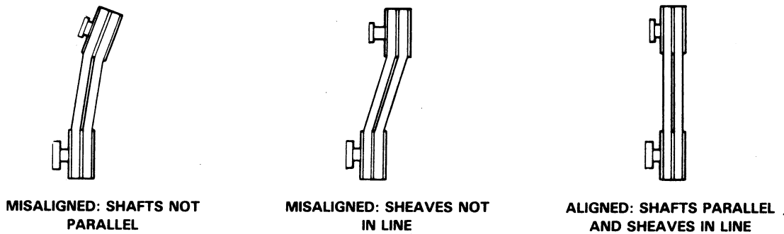
Figure 2C. Alignment of V-Belt Driven Pumps
