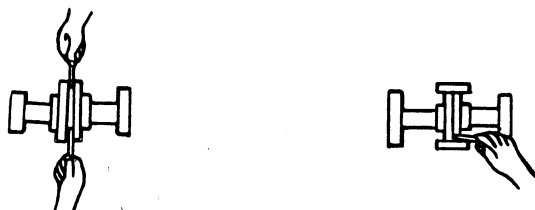
Figure 6. Aligning Non-Spider Type Couplings
