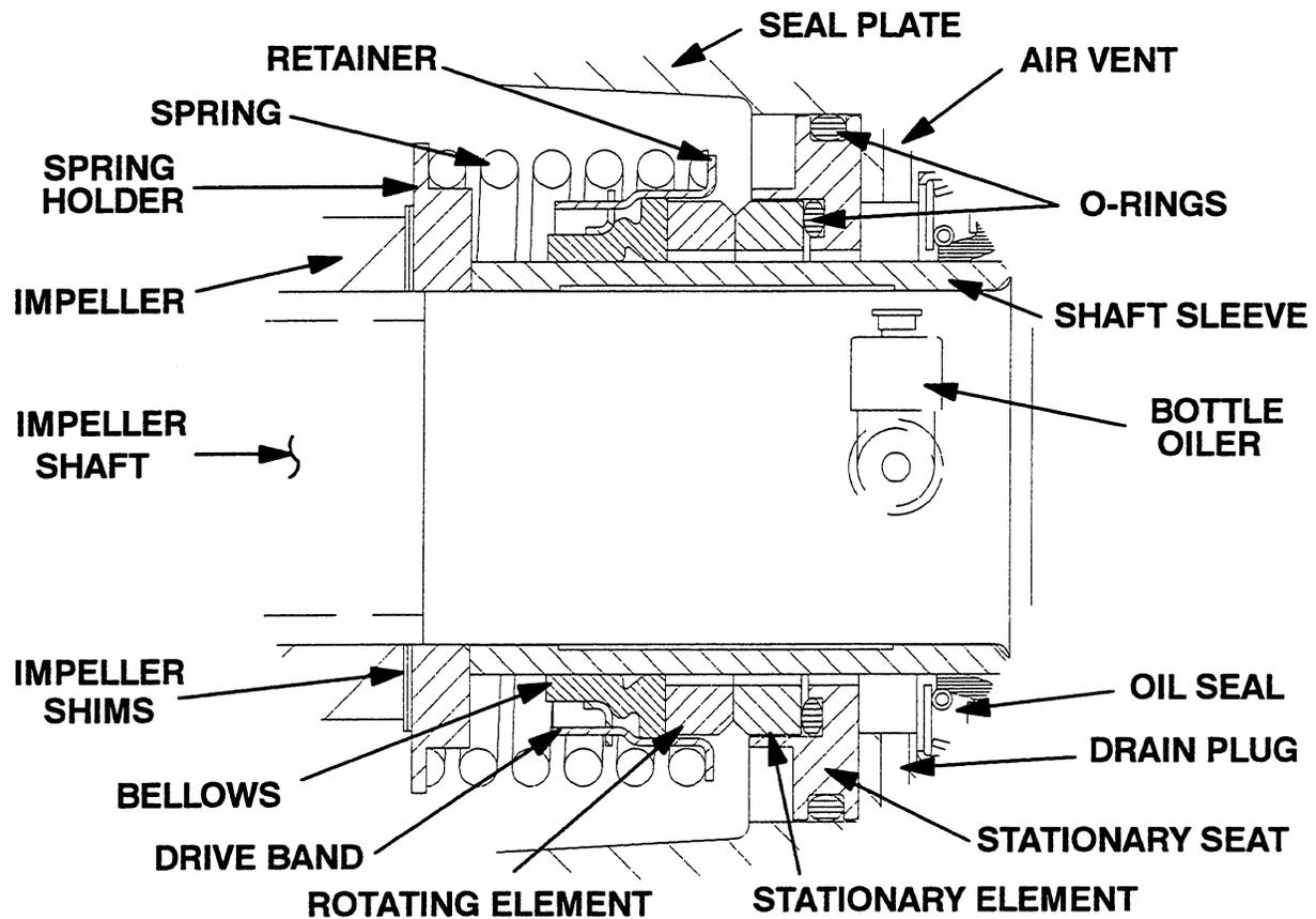
Figure 5. 12461 Seal Assembly
