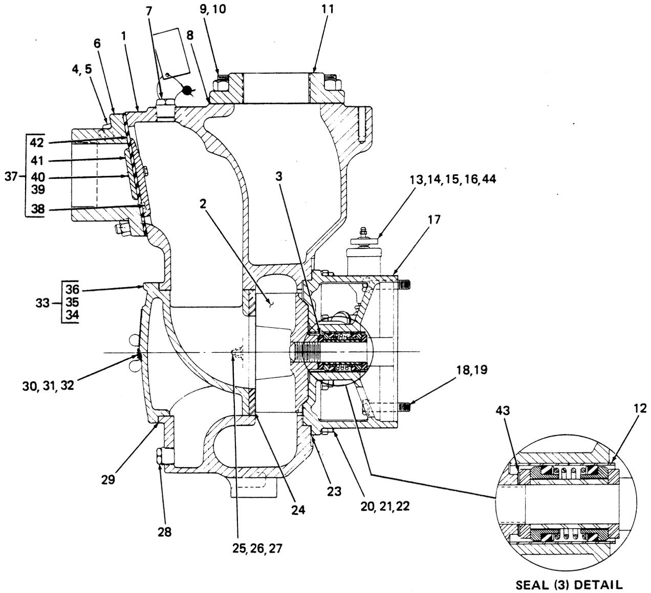
Figure 2. Pump End Only Model 13E
