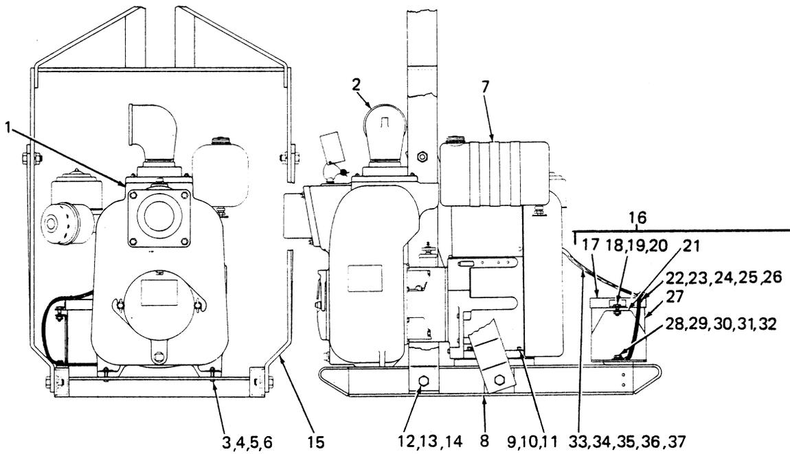
Figure 1. Pump Model 13E-S14D S/G
