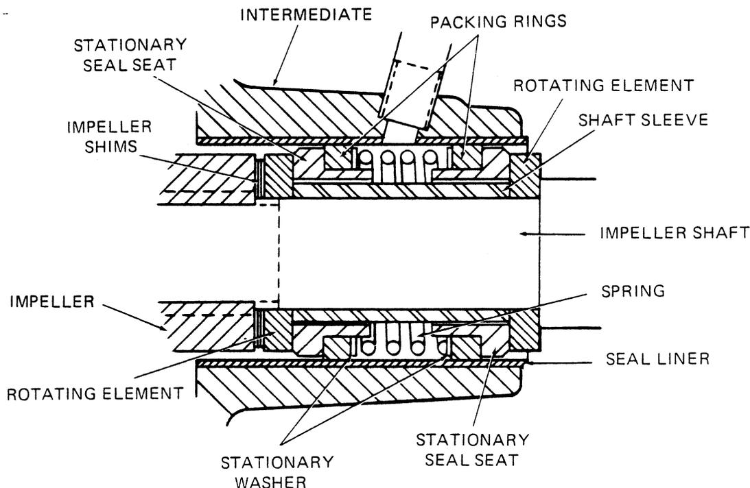
Figure 3. GS-1000-C Seal Assembly
