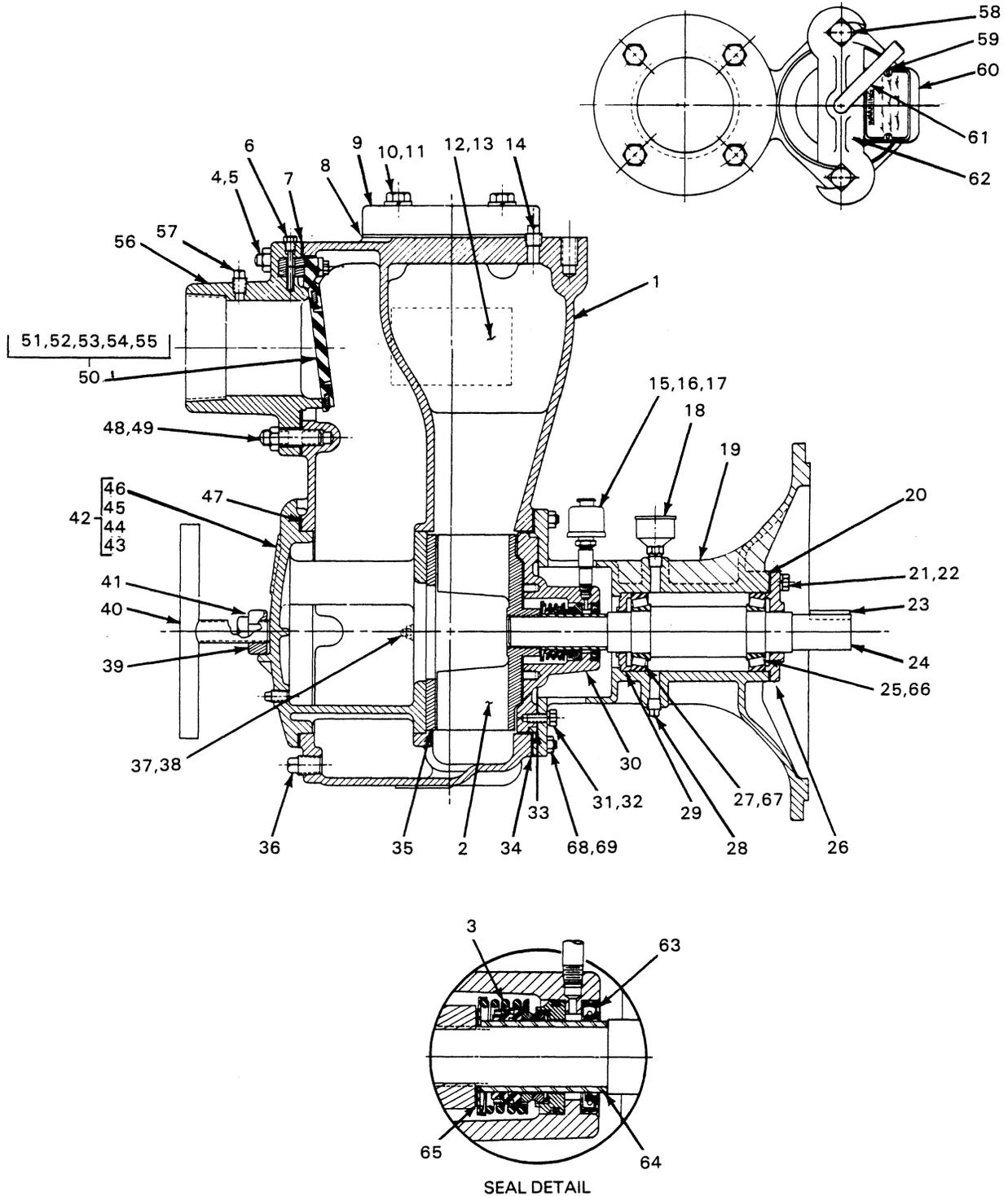
Figure 2. Pump End Assembly 14C20-F140
