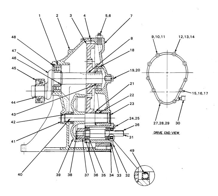
Figure 4. 44161-010 Gearbox Assembly
