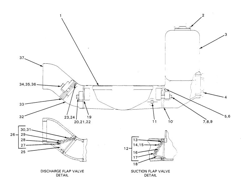
Figure 2. 46475-702 Diaphragm Pot Assembly
