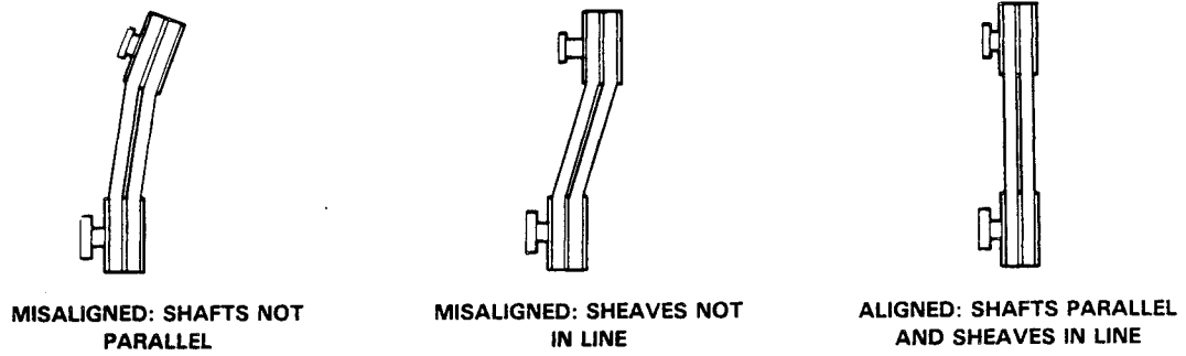
Figure 7. Alignment of V-Belt Driven Pumps
