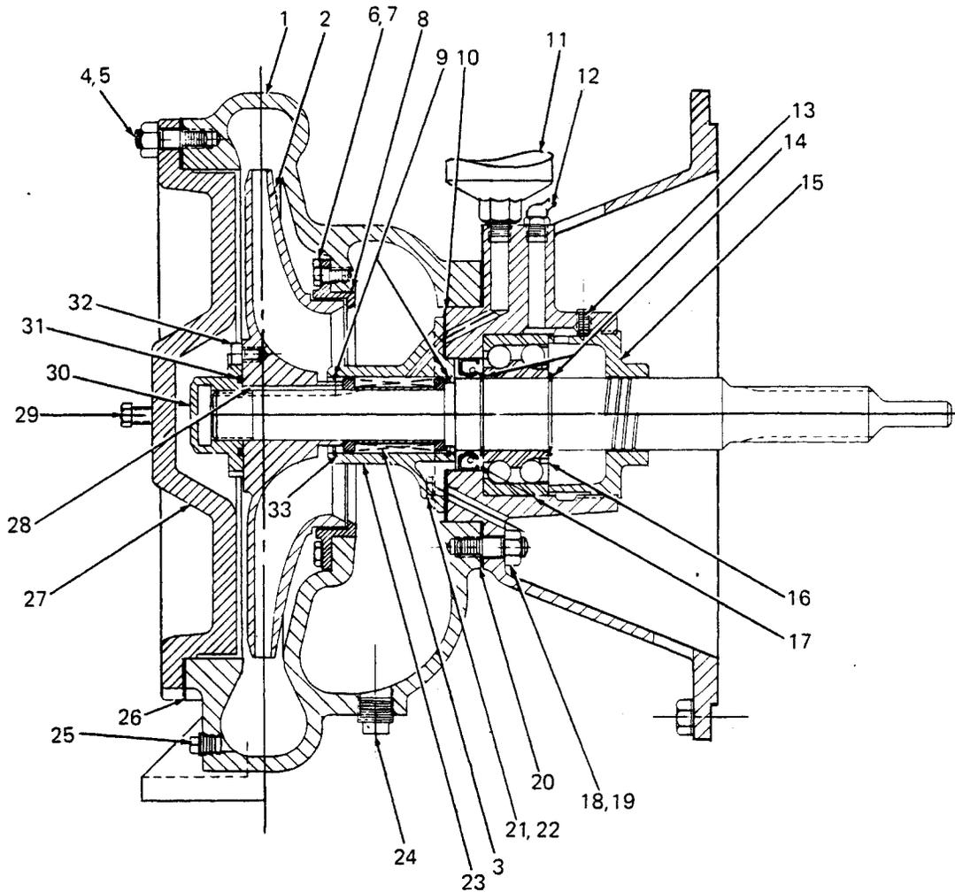
Figure 2. Pump End Only Model 54B2-F3L
