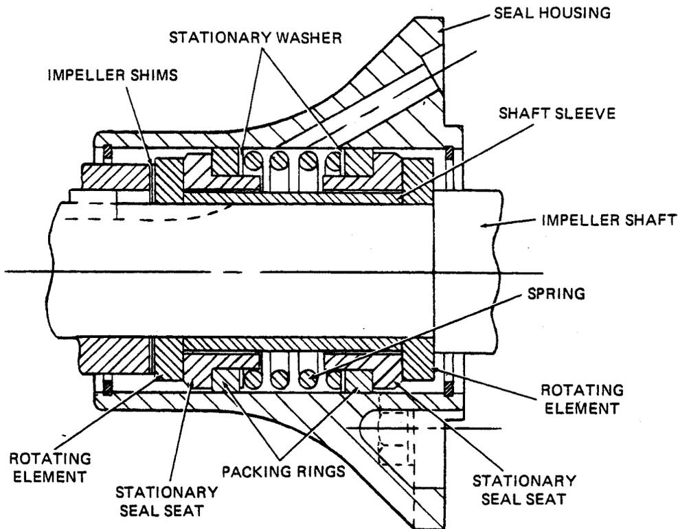
Figure 4. GS-1250 Seal Assembly
