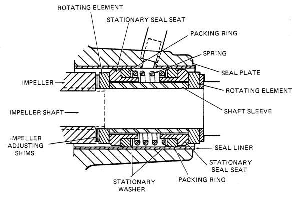
Figure 4. GS-1500 Seal Assembly
