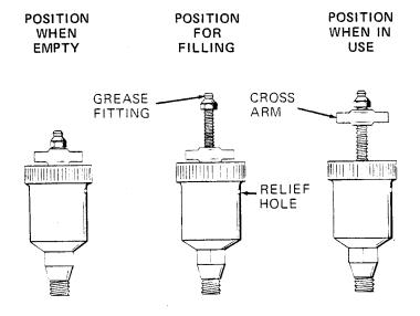
Figure 5. Automatic Lubricating Grease Cup
