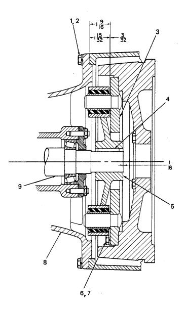
Figure 2. Pump Model 16A2-F200 Drive Assembly
